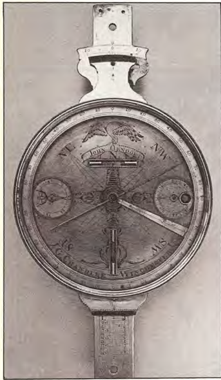
Figure 1. Surveyor's vernier compass made by Goldsmith Chandlee for John Orndorf. This particular instrument is unusual because of the additional dial and the fact that the outkeeper appears at the east point instead of at the south end of the dial plate. Also unusual is a symbolic American eagle featured at the north point. The original owner, John Orndorf, has not been identified. Photograph courtesy of Dr. Richard L. Elgin.
