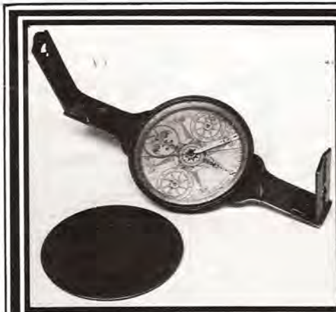
Brass surveying compass with dial cover made by Goldsmith Chandlee for J. Jackson c. 1801. Courtesy of Dale Beeks.
