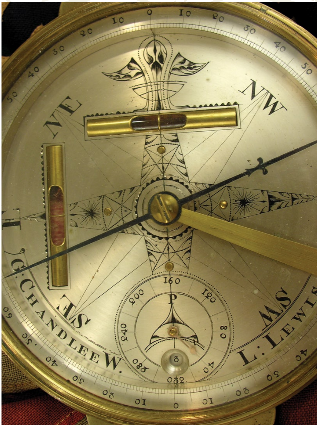
Goldsmith Chandlee engraved compass dial with inset bubble level, outkeeper dial and counter. "LT" (Links and Tenths) calculating table is engraved on the arm (see opening photo).
