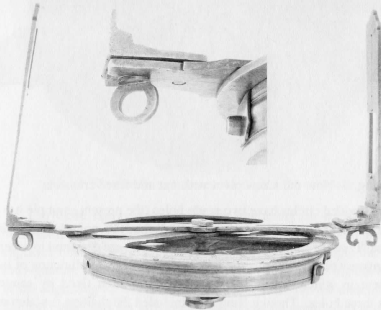
Fig. 5 Fixing screws for the sight vanes.
