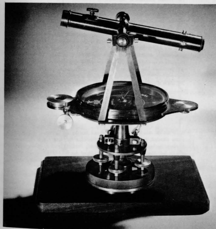
The first American Transit made by William J. Young in Philadelphia Photo Courtesy Keuffel & Esser Co. Hoboken, New Jersey
