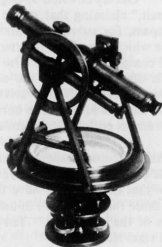
Surveyors' transit marked "Jas. W. Queen Phild a . / Warranted." While this resembles two of the known Gurley instruments, and was made by that firm, its interior details are significantly different from those of the Gurley instrument to the left. Private collection.
