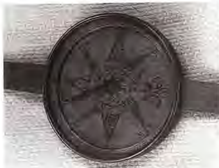
Detail view of the dial plate of the Baily surveying compass, illustrating the fine quality of engraving.
