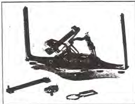
Burt's Solar Compass made by William J. Young of Philadelphia. Inscribed "Burt's Patent Made by Wm. J. Young Phil.a" on compass plate. Brass, 14 inches long, 6-1/2 inches wide, and 9-1/2 inches high. Courtesy of the National Museum of American History, Smithsonian Institution.
