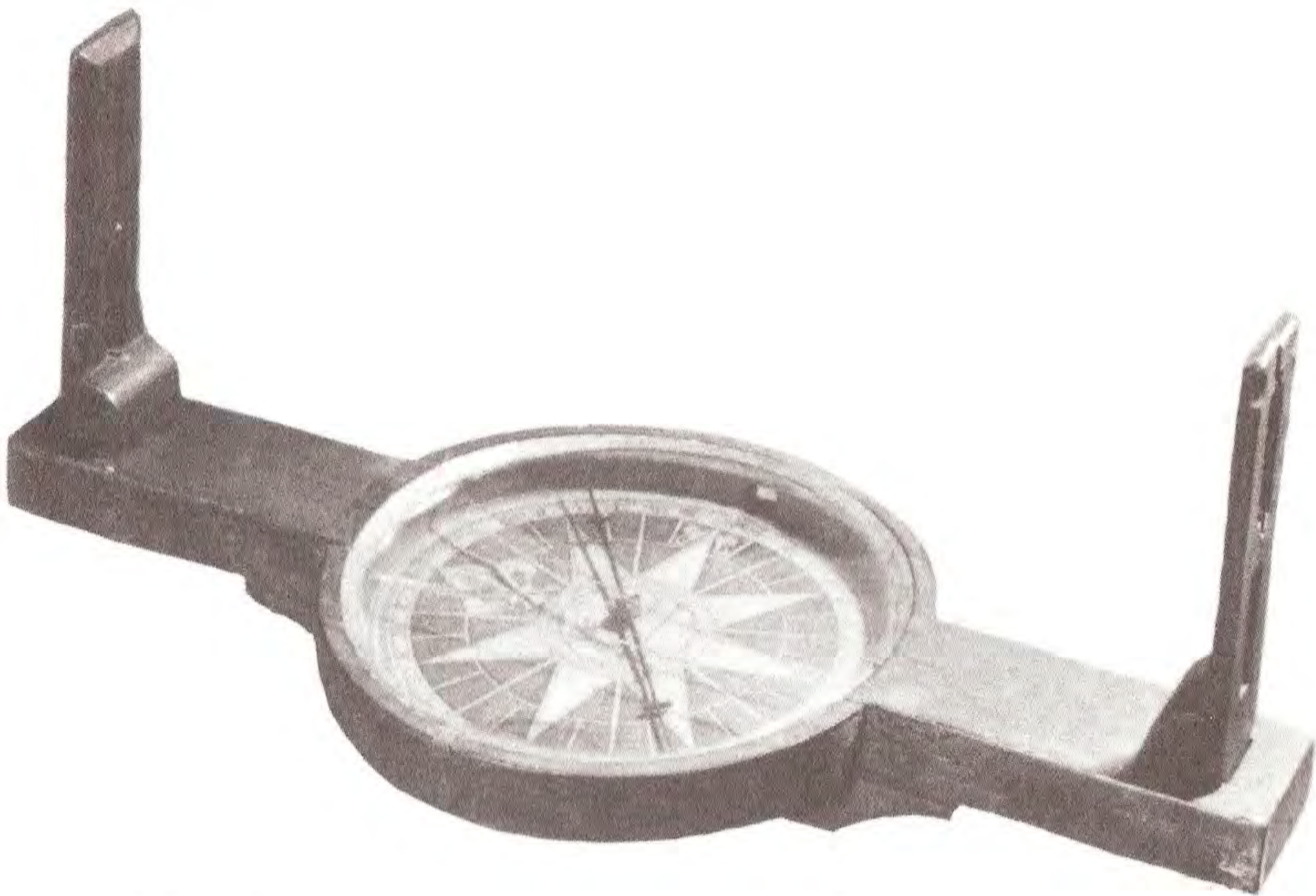
Figure 43.—Wooden surveying compass, made and sold by Thomas Greenough. The instrument is made of gumwood and has a paper compass card; it is 13\frac{1}{4} in. long and has a diameter of 5\frac{3}{4} in. In collection of Franklin Institute, Philadelphia.
