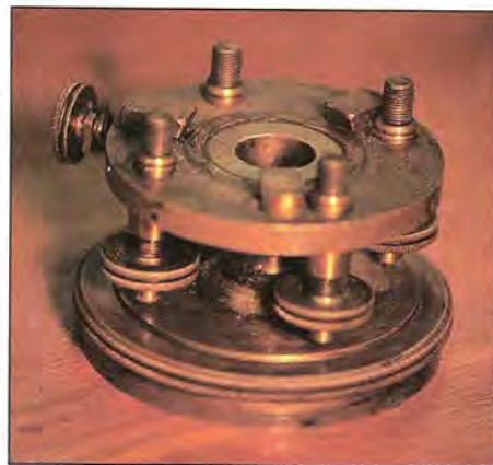
The removable lower assembly of the transit, as seen after (left) and before (above) restoration, is an unusual feature for this type of instrument and appears to be a precursor of the tribrach.
