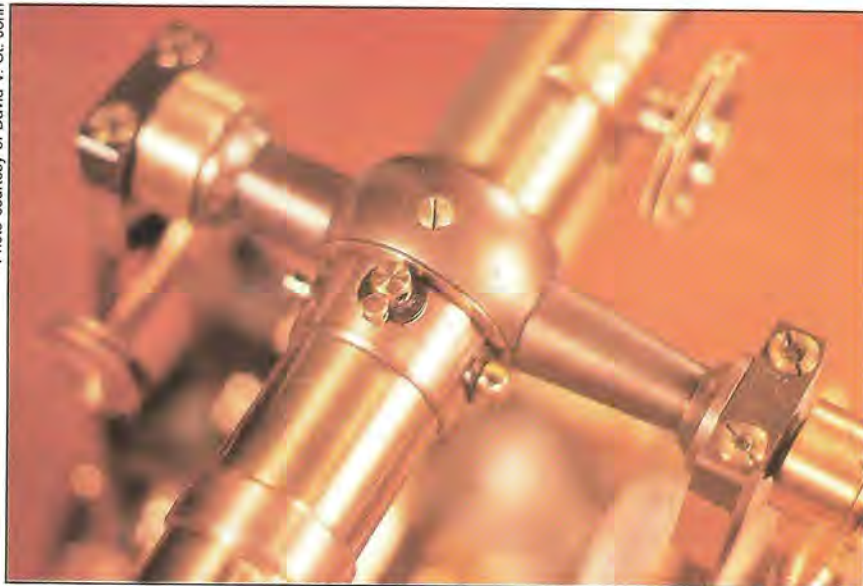
From a top view of the instrument one can see the capstan adjustment screws for adjusting the reticle and stadia. The single slotted pilot screw allows relatively quick removal of the telescope assembly for repair.
