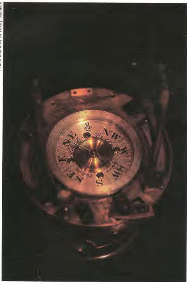
The compass plate shows the fine scrollwork and engraving—ornamentation no longer found on modern surveying instruments. The totally enclosed horizontal circle, another unique feature, did not appear on a commercial basis until the 1940s.
