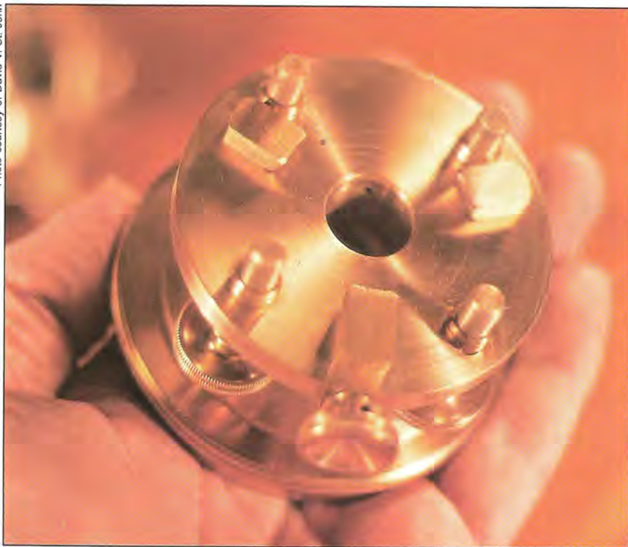
The removable lower assembly of the transit, as seen after (left) and before (above) restoration, is an unusual feature for this type of instrument and appears to be a precursor of the tribrach.
