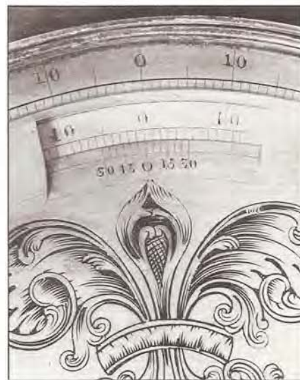
Figure 3. Detail of vernier scale above the North point of the vernier compass made by Richard Patten. Courtesy of the National Museum of American History, Smithsonian Institution.
