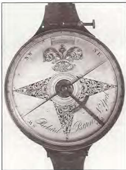
Figure 2. Detail of dial plate of vernier compass by Richard Patten. Needle is 6 inches long, the south end having a few turns of wire to compensate magnetic dip for northern hemisphere. Courtesy of the National Museum of American History, Smithsonian Institution.
