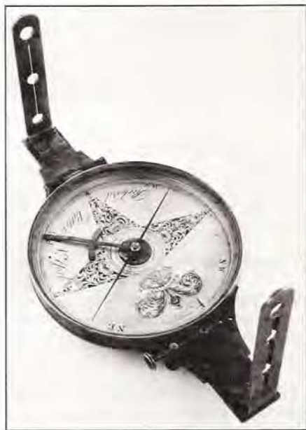
Figure 1. Vernier surveying compass made by Richard Patten of New York City. Brass, with silvered circle, dial and vernier. Single level vial. Overall length, 13 inches, width 7 inches and approximately 7 inches high. Sights detachable. Courtesy of the National Museum of American History, Smithsonian Institution.
