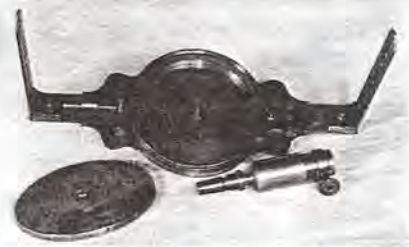
Figure 9. Surveyor's compass with a lid and toggle joint by J. Pool & Co.
