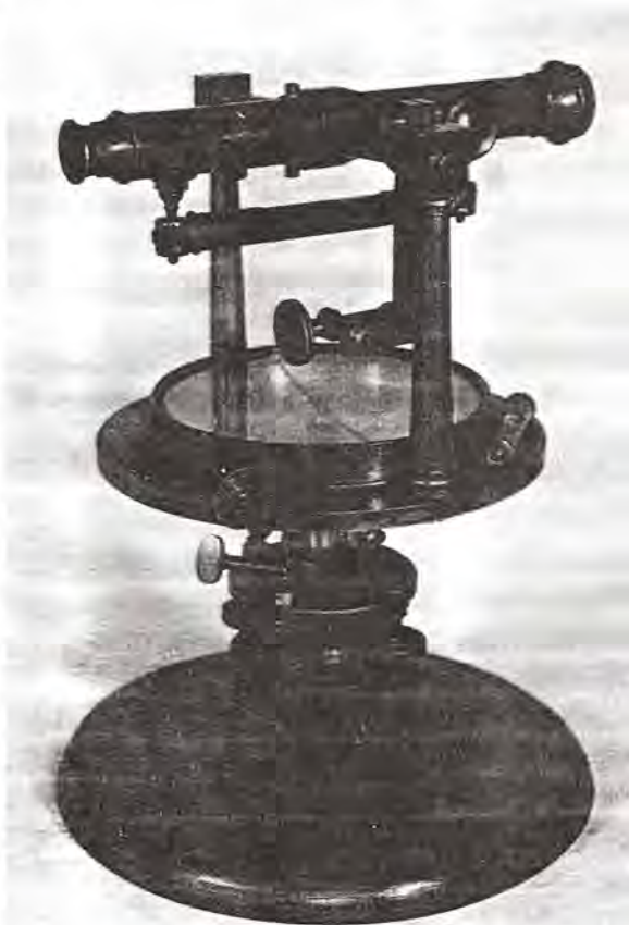
Figure 7. Compass transit on a display stand by H.M. Pool.
