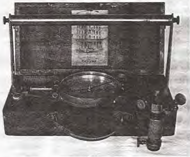
Figure 5. A surveyors compass with a sighting tube, ball and socketed head and tangent fine-screw adjustment by H.H. Pool. There is a S. Thaxter & Son trade label in the lid.
