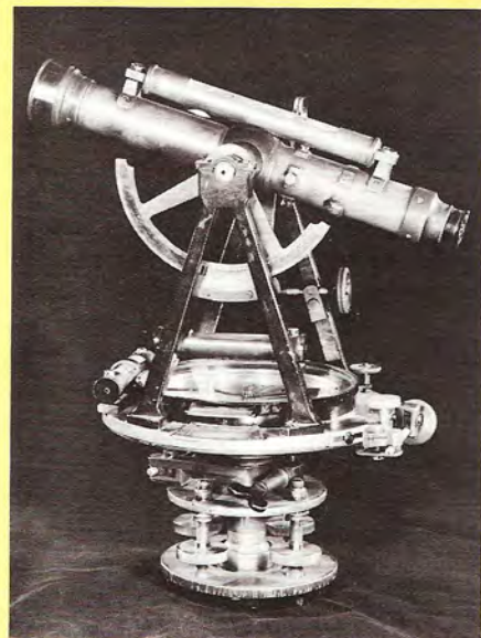
Surveyor's transit made by John Temple. Arc 5", limb 6", telescope 10-3/4", needle 4-7/16".
