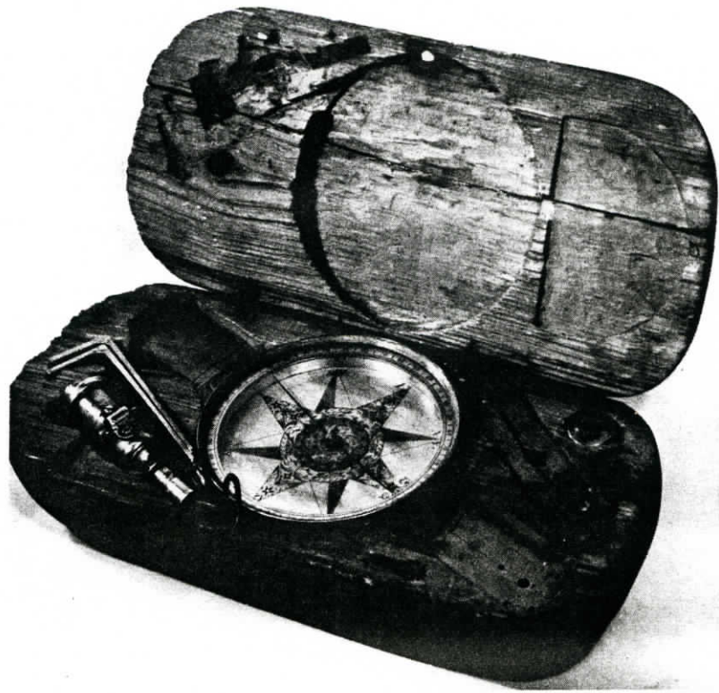
40 Vernier compass made by Benjamin Rittenhouse, with specially designed socket joint. Shown in the original field case.
