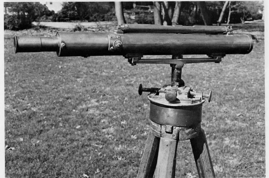
Surveyor's level signed "D. Rittenhouse". Photo courtesy of James Bean and The Historical Society of Montgomery County, Pennsylvania.
