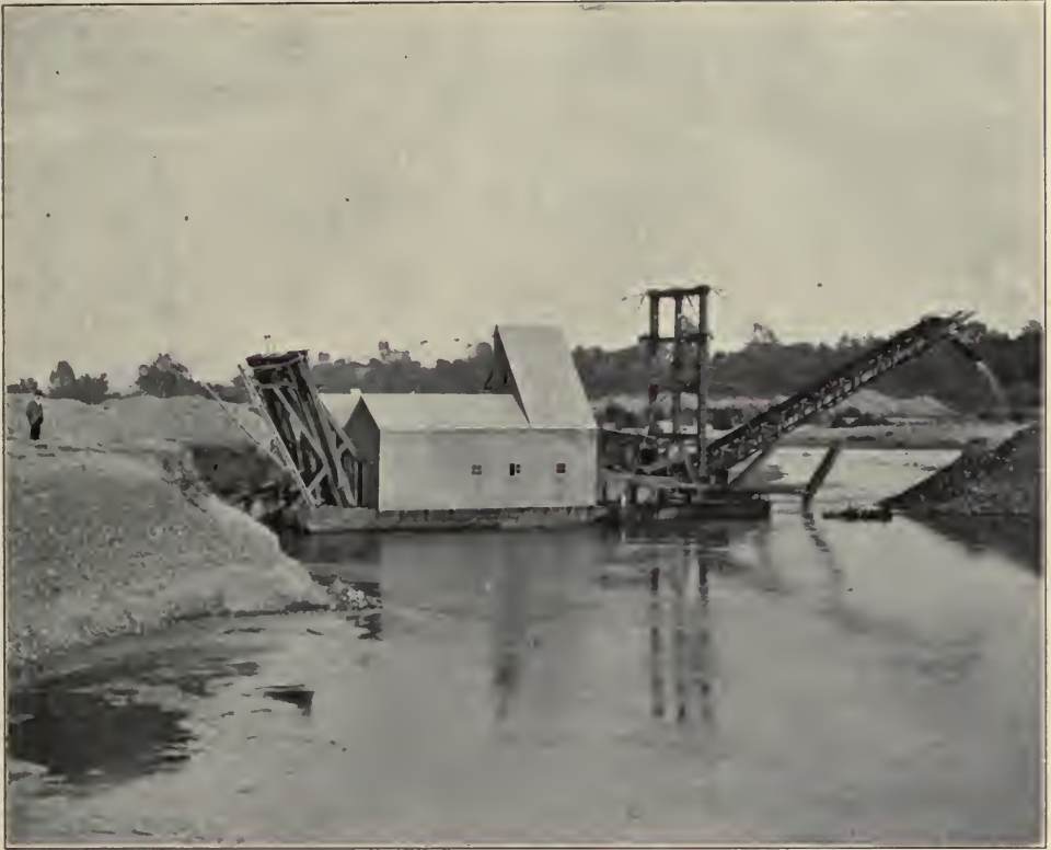
Gold dredger at work near Oroville, Butte County, California. It is claimed a fair profit is made working ground that yields five cents a cubic yard by this process
