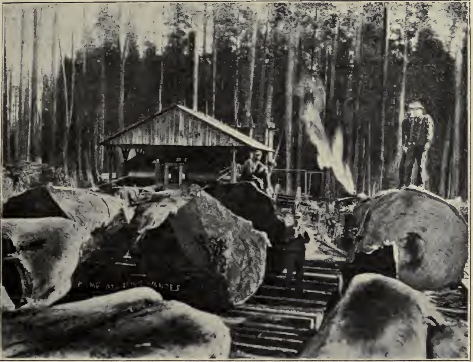
"Bull donkey" in operation at the landing on the Vance property in Humboldt County, California. The logs are hauled two miles from the timber by process of steel cables, and then transported by logging train to the sawmill at Eureka, 20 miles distant
