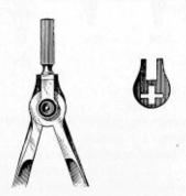
In order to prevent the compass handle from turning to either side, this improvement keeps the handle always in the center line, thus making it ready for instant use on opening, avoiding any change or correction on the compass after the exact space is once taken,
