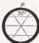
The Cross-hairs for Complete Triangulation Theodolites (N, O and P arranged for stadia work)
