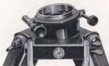
Berger (Johnson) Lower Motion (with Clamp, Tangent Screw and Opposing Spring Plunger)
