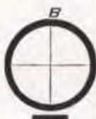
The Cross-hair Arrangements for Dumpy and Wye Levels (Diaphragms C and D are provided with Stadia hairs)
