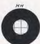
The Sun's disc, as it appears when collimated by Cross-hairs, E, F, G and H in Solar Attachments
