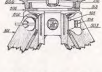
Cross Section of the Berger 18-inch Erecting Wye Level
