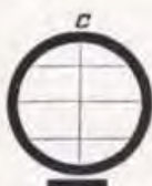
The Cross-hair Arrangements for Dumpy and Wye Levels (Diaphragms C and D are provided with Stadia hairs)
