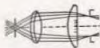
DIAGRAM SHOWING PATH OF A PENCIL OF RAYS IN AN EYEPIECE FOR AN INVERTING TELESCOPE
