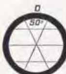
The Cross-hairs for Complete Triangulation Theodolites (N, O and P arranged for stadia work)
