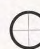
The Sun's disc, as it appears when collimated by Cross-hairs, E, F, G and H in Solar Attachments
