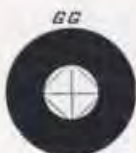
The Sun's disc, as it appears when collimated by Cross-hairs, E, F, G and H in Solar Attachments
