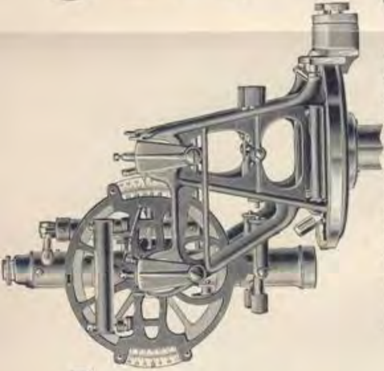
Instrument with Telescope, Vertical Circle, etc., in the Eccentric Bearings, Counterpoise attached.
