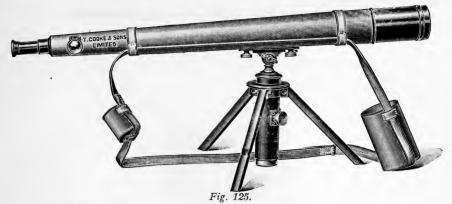
830. **TELESCOPE**, with object-glass of 3-in. aperture, power 45, taper brass leather-covered body with leather sling and caps, rack focussing motion and draw to eyepiece, on brass folding table tripod  $\pounds$  10 os. od.
