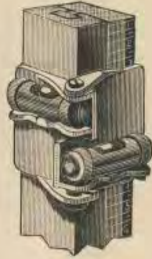
FIG. 53 C. Rod Level as applied to a Rod.
