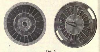
RADIALLY RIBBED AND DISHED LIMB AND PLATE, AND TAPERED CENTERS
