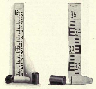
Fig. 83 Nos. 525-B to 528 Flexible or pocket leveling rods
