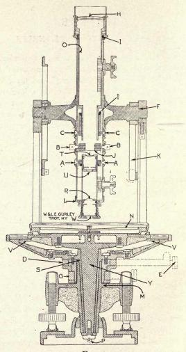
Fig. 1 Cross Section of Transit
