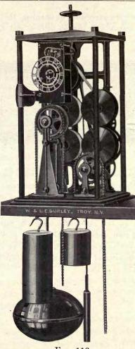
Fig. 113 No. 630 Printing Water Stage Register front view, showing clock, float and weights The type wheel indicating time is controlled by a weight driven clock of finest construction, with full jeweled escapement and compensated to endure variations of climate without variation in its regular operation.
