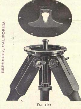
TRAVERSE PLANE TABLE MOVEMENT, SHOWING THE TRIPOD HEAD AND LEGS, THE PLUNGER CLAMP SCREW, AND THE IMPROVED SPRING BOARD PLATE The alidade consists of a brass ruler 10 inches long, graduated on the beveled edge to a scale of 40 parts to the inch, and having at each end hinged sights which fold close to the surface of the ruler. One sight has a slit and the other a hair. The alidade is furnished with a leather pouch.
