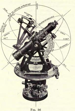
No. 30-A PRECISE TRANSIT WITH BURT SOLAR ATTACHMENT ILLUSTRATION ALSO SHOWS BEAMAN STADIA ARC be in perfect order, especially in respect to the sockets, before correct work can be done.
