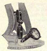
Fig. 33 No. 180 attached magnifier ATTACHED MAGNIFIERS OR MICROSCOPES are frequently used over the verniers of the horizontal or vertical limb, and are held by a universal threejointed arm, which allows the lens to be placed over any point of the vernier. The magnifier for the "A" vernier can also be used for reading the vernier of the vertical limb (any style having one vernier.)
