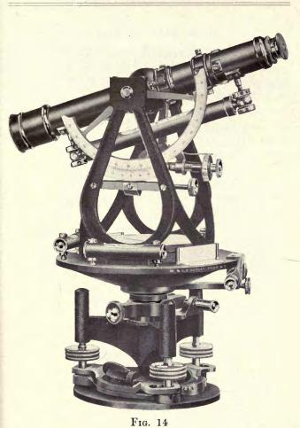
No. 10-A-3 PRECISE TRANSIT WITH THREE-SCREW LEVELING HEAD
