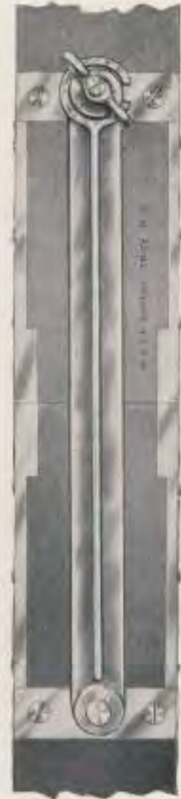
Enlarged View of Hinges, Ribbed Brace and Clamp of Telemeter Rods, Nos. 513 and 514
