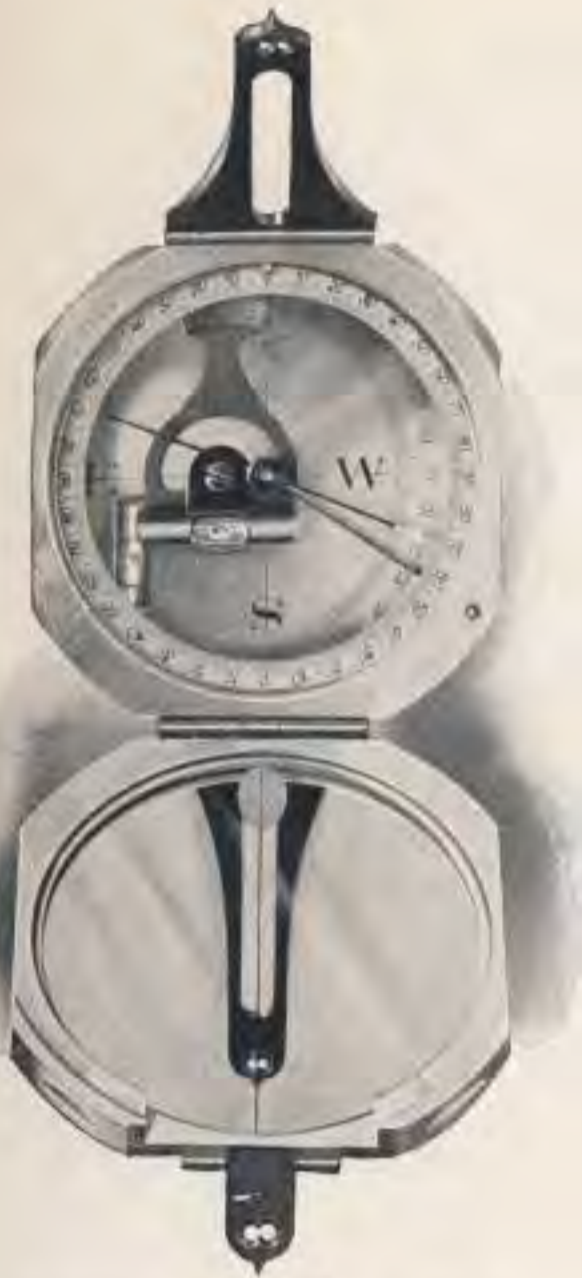
No. 3215 Brunton Pocket Transit, as used for taking courses or horizontal angles. Price $30.00
