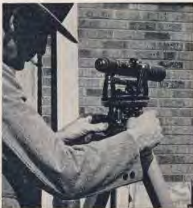
Leveling up with a cross-level on the plate, which maintains accuracy while plumbing.
