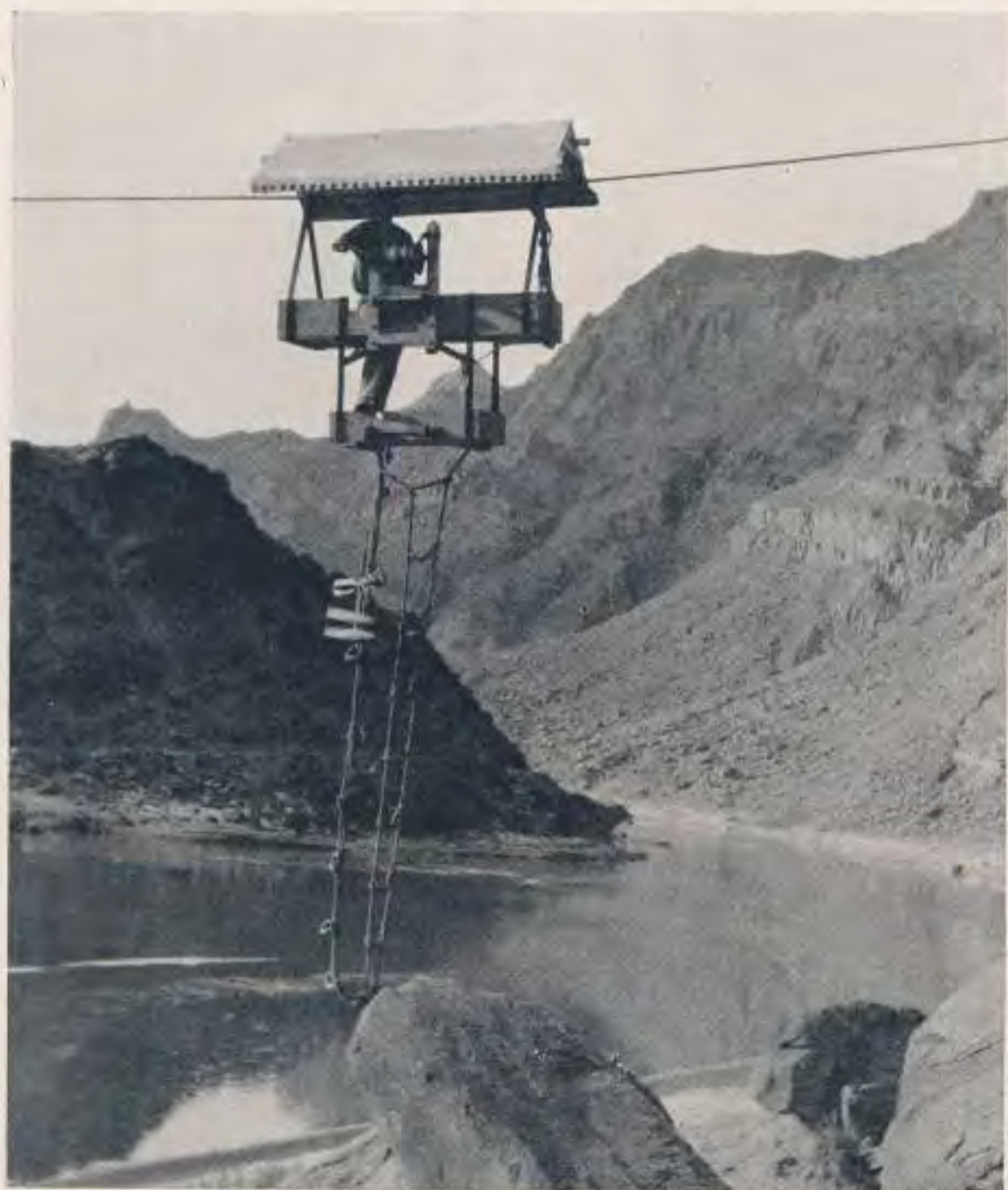
Typical Cableway with Car for Current Meter Measurements, Lees Ferry, Colorado River, Arizona. Photo Courtesy of U. S. Geological Survey.
