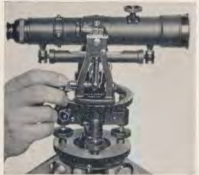
A simple turn of a slow-motion screw centers the bubble.
