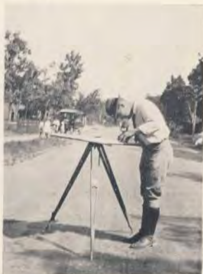
City Maps are being made in increasing numbers by the plane table method.
