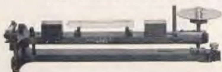
The Gurley Level Tester measures the sensitiveness and uniform running of the level bubble.
