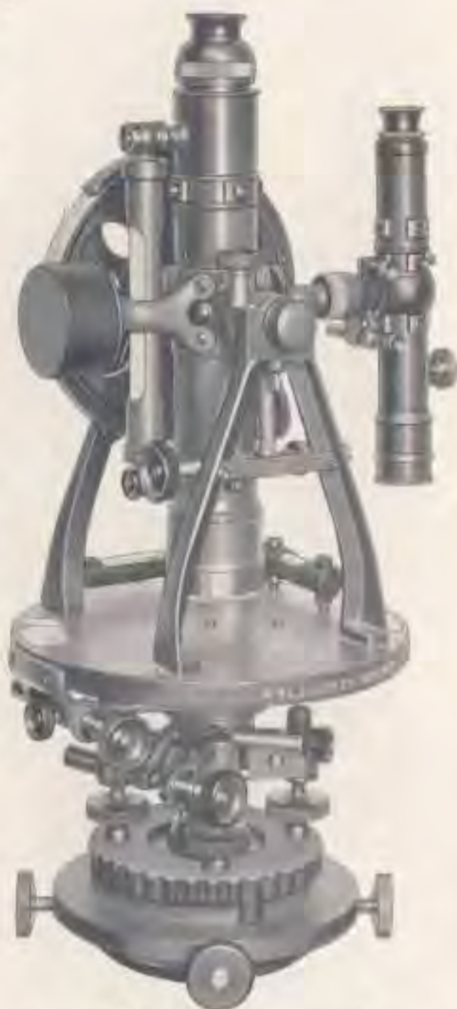
No. 137-M Mining Transit, Engineer's Model, Equipped with Rim-graduated Vertical Circle, with Guard; Auxiliary Telescope, in top position, and Micrometer Shifting Center.
