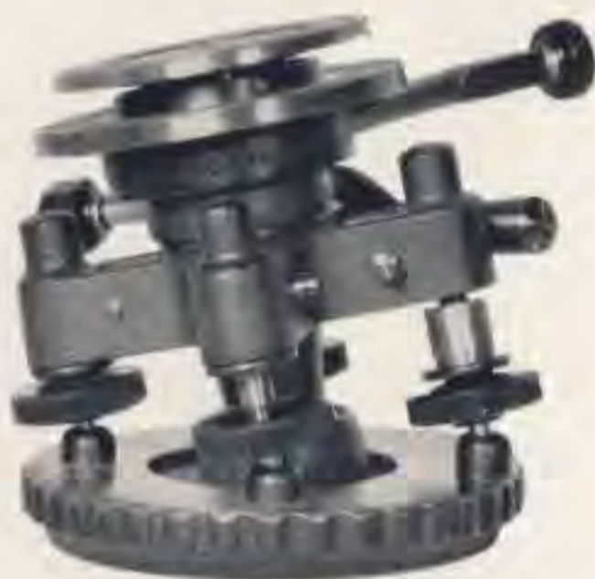
Substituting a new leveling screw and nut for a worn or jammed one is easy with new model Gurley transits. Note new screw and nut at right, ready to be slipped into the four arm piece.
