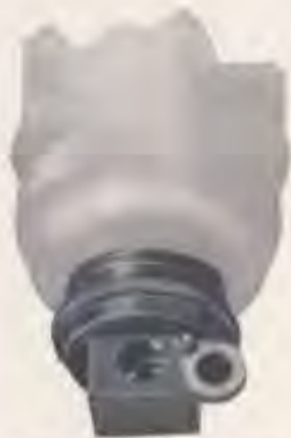
Diagonal Prism attached to the Eyepiece of a Transit
