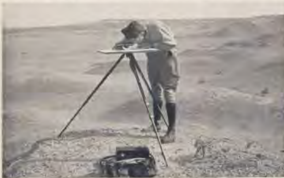
On the Third Asiatic Expedition of the American Museum of Natural History, the Topographer used a Gurley Explorer's Plane Table Outfit. It was on this expedition that the dinosaur eggs were discovered.
