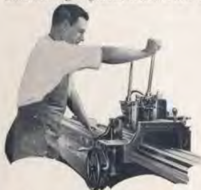
Stamping the graduations into Gurley Leveling Rods.
