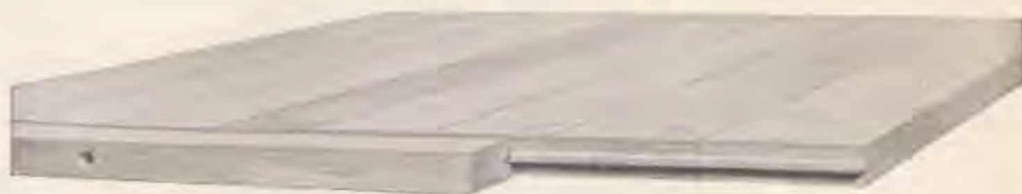
Cross-Section of Gurley Plane Table Board
