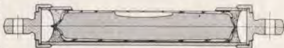
Cross-section of level vial mounted in case.
