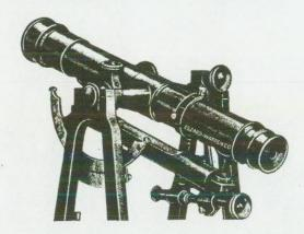
The Vertical Arcs are of  $2\frac{1}{2}$ " radius, and swing freely in bearings on the telescope axle, so that they can be set and clamped at zero, regardless of the position of the telescope. This feature is peculiar to Vertical Arcs of Transits of our make and is of great value to the Engineer.
