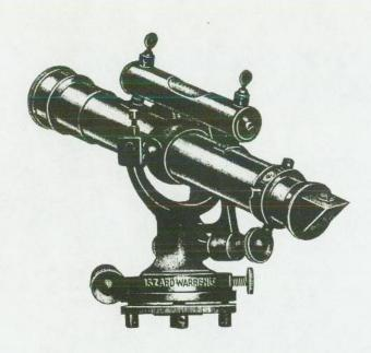
The Solar Attachment consists of a small telescope that is mounted on a horizontal axis, resting upon a standard connected to a circular base. This base forms the socket of the, so called, polar axis and is attachable at its lower extremity to the horizontal axis of the telescope. The solar telescope is thus capable of being turned on its own horizontal axis and on its polar axis. A small level is mounted on top and parallel to the solar telescope.
