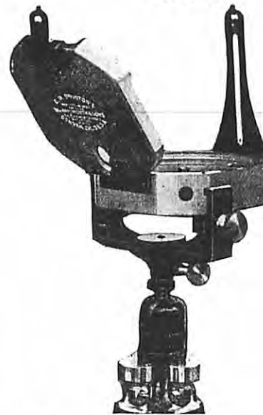
Showing Brunton Transit on Ball and Socket Tripod Head No. 185C.
