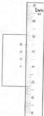
Illustrating graduation of vertical arc, vernier reading to minutes.
