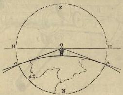
In the above diagram, A a represents a portion of the earth's surface, and O the place of an observer; H O H will be his true horizon, O A and O a his visible horizon; these rays being tangents to the earth's surface at A and a; the angle, H O A, or H O a, is the dip of the horizon, which it is the business of the dip-sector to measure. But the arcs to be
