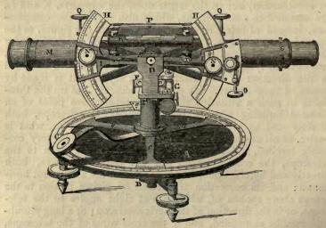
The horizontal circle (or limb), A, of this instrument consists of one plate only, which, as usual, is graduated at its circum-
