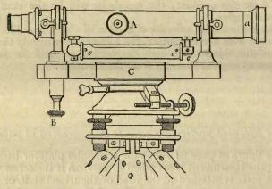
The above figure represents this instrument; it has an achromatic telescope, mounted in Y's like those of the theodolite, and is furnished with a similar system of cross wires for determining the axis of the tube, or line of collimation. By turning the milled-headed screw, A, on the side of the telescope, the internal tube, a, will be thrust outwards, which carrying the object-glass, it is by this means adjusted to its focal distance, so as to show a
