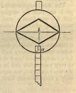
The line on the bevelled edge at a (as before stated) denotes the reading of the staff; therefore, a piece equal in length to the distance, a b, is cut off from the bottom of the staff, or rather the divisions commence at that number of inches above 0.
