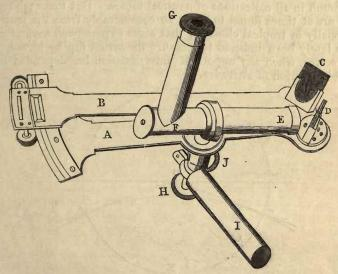
The preceding figure represents this instrument: A is the sector, B the index, with its clamp and tangent-screw, exactly similar to that of the sextant: the index-glass, C, and the horizon-glass, D, are fixed at right angles to the plane of the instrument. The telescope, E F, is fitted into a collar, having an up-and-down motion given to it by turning the screw H; the
