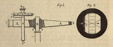
The divisions on the graduated circle indicate spaces of five minutes each, which are read off along with the degree, by means of an index-pointer. The remaining minutes and seconds, if any, are determined by the reading microscope, as was stated when describing the construction of the circle; it now remains
