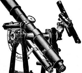
C. L. Berger & Sons' Latitude Level Attachment. Shown as applied to a Transit with Solar Attachment.
