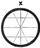
Diaphragm showing arrangement of wires as used with our mine transits, to distinguish center horizontal wire from stadia wires, to avoid mistakes.
