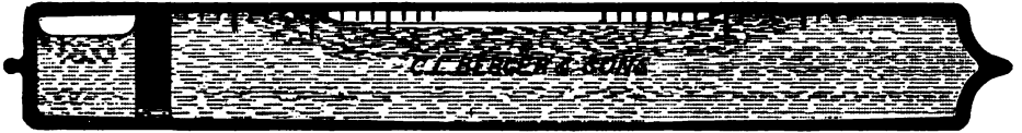
Cross-section of spirit levels as above, but provided with an air-chamber for adjusting length of the bubble for different temperatures as used in the leveling instruments of precision and for astronomical work.
