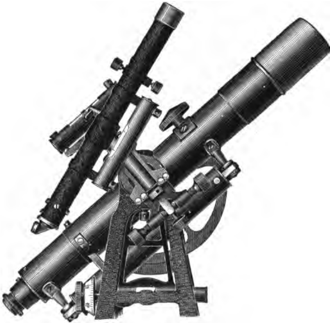
Surveyors' Solar Attachment.
