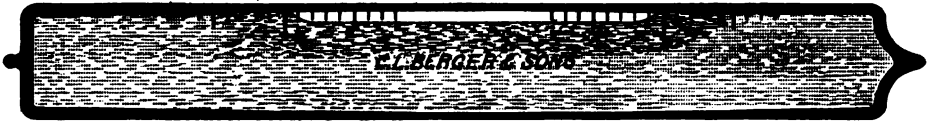
Cross-section of spirit levels as used for instruments of precision (see pages 7 and 38), interior surface showing the barrel form with curvature ground to certain value of arc, diameter of arc depending on the degree of sensitiveness required.
