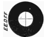
The Sun's disc, as it appears when collimated by wires E, F, G and H in Davis's Solar Attachments. (See pages 81 and 174.)
