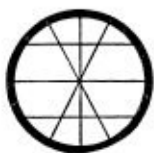
Special Stadia hair arrangement for triangulation work, furnished special on our instruments, or can be supplied separately
