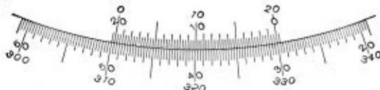
Fig. 3. Circle divided to 20 minute spaces, vernier reading to 20".
