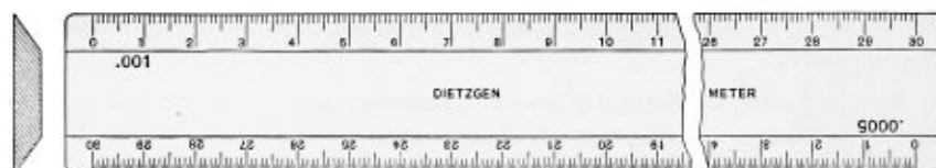
No. 1460. 10 cm. long, divided mm. \times half mm.
