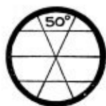
Special Stadia hair arrangement for triangulation work, furnished special on our instruments, or can be supplied separately
