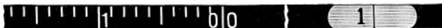
Graduations of the extra subdivided foot before the zero on the Empire Chain Tape
