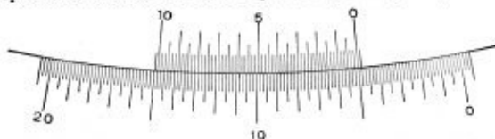
Fig. 4. Circle divided to 10 minute spaces, vernier reading to 10".
