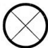
Special Stadia hair arrangement for triangulation work, furnished special on our instruments, or can be supplied separately
