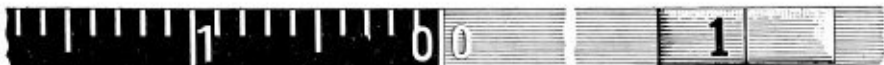
Graduations of the extra subdivided foot before the zero on the Indestructible Chain Tape
