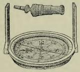
This little instrument, shown with jacob staff socket in fig. 17, though not used in extensive surveys like the larger compasses we have described, is found very convenient in making explorations, or in retracing the lines of government surveys, as in locating land warrants, &c.
