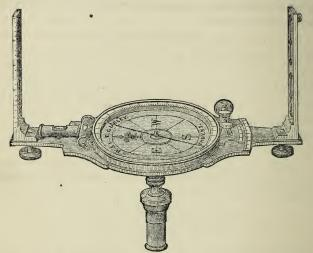
The Vernier Compass, represented in fig. 2 differs from the instrument just described, in having its compass circle with a vernier attached, movable about a common centre, by turning the "tangent screw," seen at the south end of the plate.
