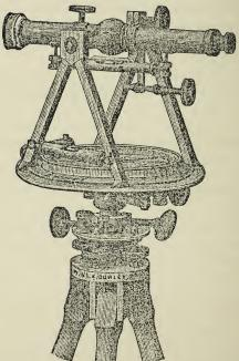
The Surveyors' Transit, of which the above cut is a representation, is in principle, very similar to the instrument just described, differing from it mainly in the substitution of the telescope with its appendages, for the ordinary compass sights. THE TELESCOPE is of somewhat finer quality than that used with the Vernier Transit; as here shown, it is furnished with a small level, having a ground bubble tube and a scale; sometimes. also a vertical circle is connected with its axis.
