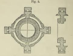
THE CROSS-WIRES.—The cross-wire diaphragm, two views of which are here exhibited, is a small ring of brass, suspended in the tube of the telescope by four capstan head screws, which press upon the washers shown on the outside of the tube.
