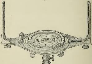
As shown in Fig. 10, this instrument has the main plate, levels, sights, and needle of the ordinary instrument, but is also provided with a circle on the outside of the compass box, divided all around and reading by two opposite verniers to single minutes of a degree.
