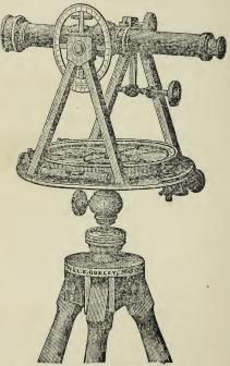
The Vernier Transit, or Transit Compass, represented in the cut above, has the same general properties as the Vernier Compass, but is furnished with a telescope in place of the ordinary sights. The telescope is from ten to twelve inches long, and sufficiently powerful to see and set a flag at a distance of two miles, in a clear day.
