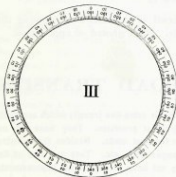
III Horizontal limb, numbered 0-360 and in quadrants.
