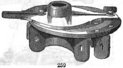
259. Saxe's Patent adjustable Tripod head, with a movement of 2½ inches, enabling the Engineer or Surveyor to adjust his instrument over any given point, without moving the Tripod legs or unscrewing the levelling screws. This is so readily accomplished that it makes this adjuster far superior to any heretofore constructed.
