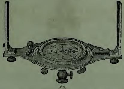
The Railroad Compass has the Main Plate, Levels, Sights and Needle of the ordinary Surveying Compass, but has also underneath the main plate a divided circle or limb by which horizontal angles to single minutes can be read independently of the needle.
