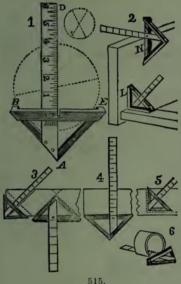
This square combines, in a most convenient form, five different instruments, viz., The TRY-SQUARE, the MITER, the T-SQUARE, the GRADUATED RULE, and (what is entirely new) the CENTRE-SQUARE, for finding the centre of a circle.
