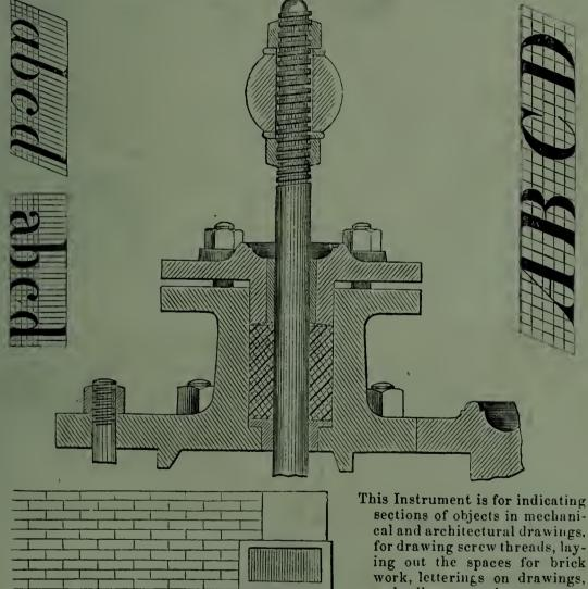
cal and architectural drawings, for drawing screw threads, laying out the spaces for brick work, letterings on drawings, and all cases where narrow spaced parallel lines are needed. With it, a person of moderate ability or practice can produce an effect of uniformity and neatness, in sectional drawings, almost, or quite equal to the engine dividing of engravings. The instrument consists
