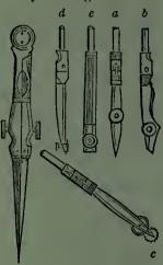
Another form of the pocket dividers is so constructed as to include points for per and pencil, and yet, all contained in a very small compass. No. 79 represents this
