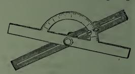
machinists, in obtaining or laying off bevels upon a viece of machinery.
