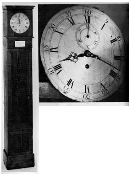
Figure 6.—Astronomical clock made by David Rittenhouse for his observatory at Norristown, Pa., and used by him for the observation of the transit of Venus in 1769. Unembellished pine case 83-1/2 in. high, 13-1/4 in. wide at the waist with a silvered brass dial 10-5/8 in. diameter. Photo courtesy the American Philosophical Society.
