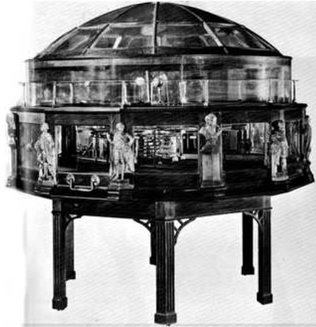
Figure 18.—Orrery by Joseph Pope completed in 1787 for Harvard University. Engraved plates and bronze figures were made by Paul Revere. The orrery is 6-1/2 ft. in diameter and 6-1/2 ft. high. The twelve figures at the corners are said to have been carved in wood by Simeon Skillin and cast in bronze by Paul Revere. Photo courtesy Harvard University.
