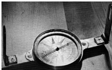
Figure 42.—Brass surveying compass made by Thomas Greenough (1710-1785) of Boston. Compass face is mounted on main blade with two copper rivets. Screws for vanes and tripod mounting are hand cut, with wing nut ends. Sighting bars are 1/16 in. wide and 5-1/4 in. high; over-all length is 11-7/8 in. and diameter is 5-1/4 in. Owned by Greenough family of Boston. Photo courtesy of Dr. Thomas Greenough.
