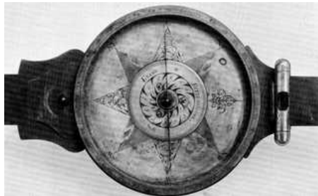
Figure 81. —Brass surveying compass marked "Rittenhouse & Evans," about 1780. Over-all length, 13-3/4 in.; diameter of dial, 5-1/4 in. This instrument, made about 1780, was owned and used by John Johnson in 1818 for surveying the boundaries between Canada and Maine. USNM 309543.
