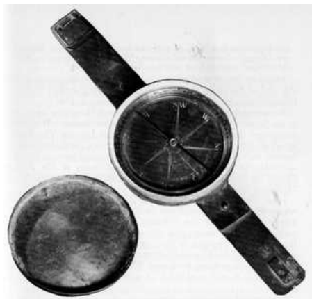
Figure 17.—Brass surveying compass made by Stephen Greenleaf (fl. 1745) of Boston. Photo courtesy New Hampshire Historical Society, Concord.
