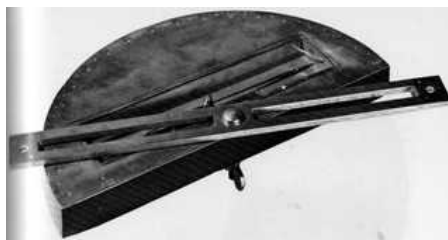
Figure 34.—18th-century semicircumferentor. Inscribed brass plate is mounted on a mahogany block; brass sighting bars are mounted on a swivelling bar. The trough compass is on a silvered dial. In collection of the writer.
