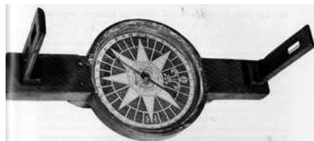
Figure 41.—Wooden surveying compass made by James Halsy (1695-1767) of Boston. The instrument is 11 in. long. In collection of East India Marine Hall, Peabody Museum, Salem, Massachusetts.
