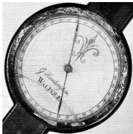
Figure 66.—Views of wooden surveying compass made by Gurdon Huntington, clockmaker in Walpole, New Hampshire, between 1789-1804. Made of cherry with folding brass sighting bars, the instrument is 14 in. long and 5-1/2 in. wide. In collection of the writer.
