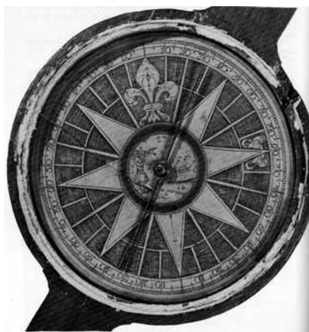
Figure 46.—Compass card from a wooden surveying compass "Made by Thomas Greenough, Boston, New England." In collection of the writer.
