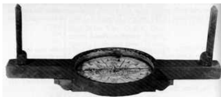
Figure 61.—Wooden surveying compass made by Benjamin Warren (c. 1740-c. 1800) of Plymouth, Massachusetts, and detail of the compass card. The compass, made of cherry wood, is 12 in. long and has a diameter of 6 in. In Streeter Collection of Weights and Measures, Yale University.
