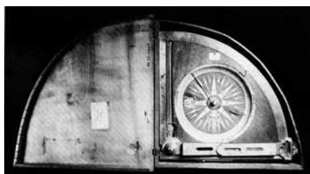
Figure 69.— Wooden surveying instrument inscribed "Invented by P. Merrill, Esq." and "Made by John Kennard, Newmarket." Made of walnut, 7-3/4 in. long; in its original pine case, with cover. The compass card and dial (see opposite) were made by Thomas Salter Bowles of Portsmouth. In Frank C. Churchill Collection, Dartmouth College Museum, Hanover, New Hampshire.
