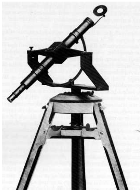
Figure 31.—Equal altitude telescope, 17 in. long, made and signed by Henry Voight (1738-1814) of Philadelphia. USNM 311772.
