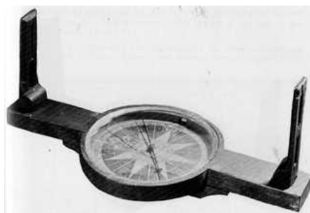
Figure 43.—Wooden surveying compass, made and sold by Thomas Greenough. The instrument is made of gumwood and has a paper compass card; it is 13-1/4 in. long and has a diameter of 5-3/4 in. In collection of Franklin Institute, Philadelphia.
