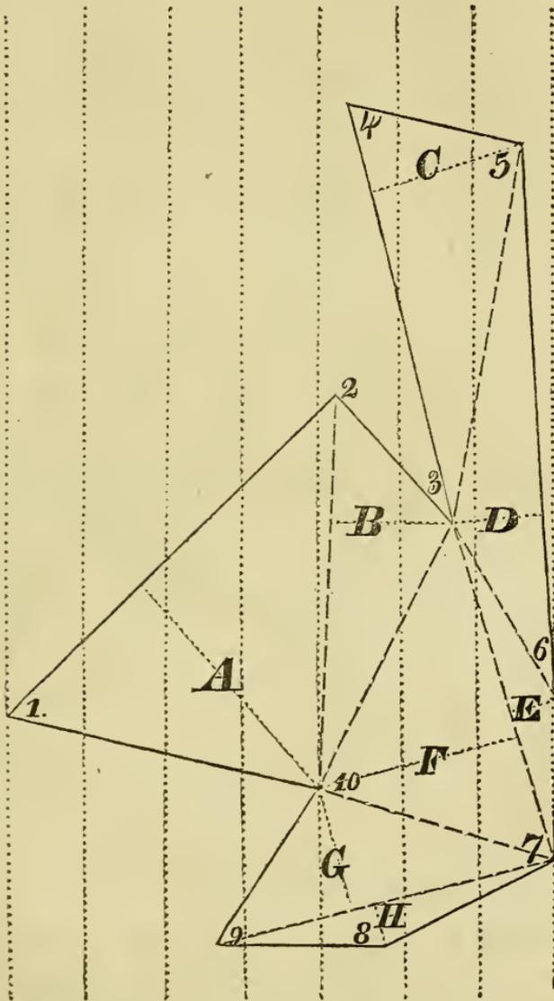
Plot of a survey, wherein the area is cast up by reducing the whole survey of a *single triangle*. This is referred to and explained from sections 96 to 99.
