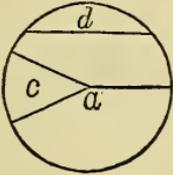
*Circle*, is a figure bounded by a continued line, every where equi-distant from a point in the centre. *c* sector, bounded by two radii and an arc; *d* segment, bounded by a chord line and an arc; *a* the centre.
