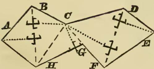
Field surveying with a cross, where a farmer is desirous to know the contents of a field for planting seed, to pay for mowing by the acre, &c. See sec. 60 and 61.
