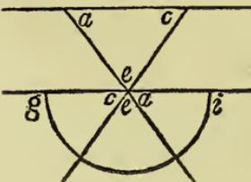
Illustration of the principle that a triangle contains 180 degrees. Semi-circle  $g i$  is the measure of  $180^\circ$ —angle  $a$  in it equals angle  $a$  in the triangle— $e$  equals  $e - c$  equals  $c$ . Sec. 33, article 5.
