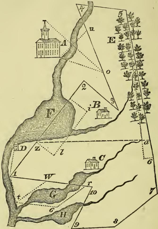
Plot of a survey referred to from sections 91 to 95 ; wherein the method of reducing and raising the scale, plotting, *triangular cuttings* and *castings* are explained.
