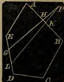
As before, compute the area,  $AEGH$ , subtract it from  $mc$ , the difference is the difference between the triangles  $PGL$  and  $PHK$ . Draw  $PKL$  the line that divides the polygon as required.
