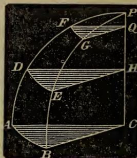
Observe that  $DE$ ,  $FG$ , &c., are parallels of latitude, that is, they are parallel to  $AB$ , the plane of the equator.
