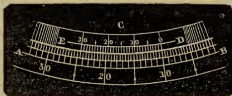
In case 0 on the vernier makes a right line with  $10^\circ$  on the arc as is represented in the figure, then the index marks  $10^\circ$ . But if 0 on the vernier is a little beyond  $10^\circ$  we then look along the vernier
