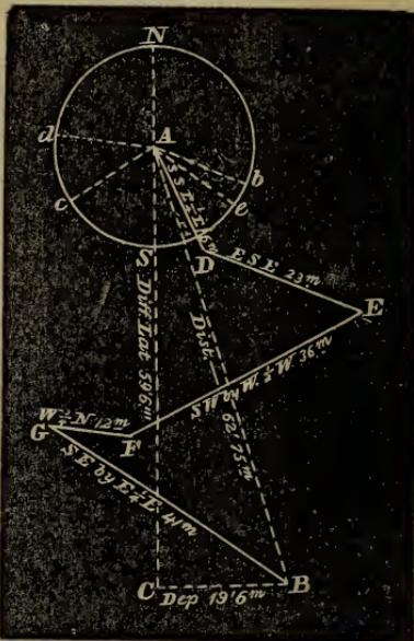
\* Two and  $\frac{1}{4}$  points is  $25^\circ 18' 45''$ , that is, take the chord of  $25^\circ 18'$  in the dividers, and set it off from  $s$  to  $a$ , and so on, for other angles.
