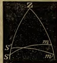
Here are two distinct triangles,  $ZS'm'$ , and  $ZSm$ . The apparent altitudes subtracted from  $90^\circ$ , give  $ZS'$  and  $Zm'$ , and  $S'm'$  is the *apparent distance*; with these three sides, the angle  $Z$  can be found. Correcting the altitudes, and subtracting them from  $90^\circ$ , will give the sides  $ZS$  and  $Zm$ ; these two sides, and their included angle at  $Z$ , will give the side  $Sm$ , which is the *true distance*.
