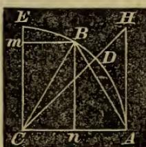
and the sides opposite to equal angles are equal; that is,  $AB$ , the chord of  $60^\circ$ , is equal to  $CA$ , the radius.
