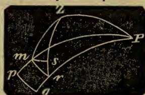
altitude, and  $pq$  the measure of the required error in time. And as the sides of the triangle  $msr$  will necessarily be small, that triangle may be considered as a rectilinear one, right angled at  $s$ ; and because the angle  $Prm$  is also a right angle, the angles  $smr$  and  $PrZ$ , being each the complement of  $mrs$ , are equal to each other
