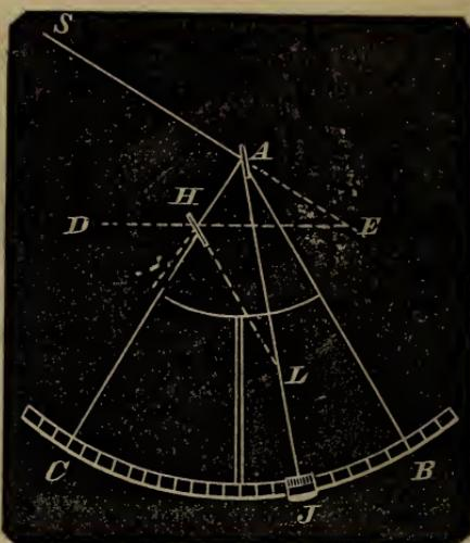
the interior opposite angles ; therefore, by the *preceding lemma*, the angle  $HLA$  is half the angle at  $E$ , but as  $AB$  and the mirror  $H$  are parallel, the angle  $HLA$  is equal  $JAB$ . It is obvious that  $JAB$  is measured by the arc  $BJ$ , or it measures the angle at  $E$ , if half degrees on  $BC$  are counted as whole ones, which was to be shown.
