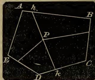
When the whole is to be divided into four parts, in the ratio of  $m, n, p, q$ , then draw  $hk$ , so that one portion shall be ( $mc+nc$ ) and the other ( $pc+qc$ ).
