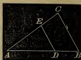
Which shows that if we have the numerical value of  $AB$ , and of  $n$  and  $m$ , we can find that of  $AD$ , and from  $D$  draw  $DE$  parallel to  $BC$ , and the triangle is divided as required.
