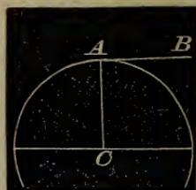
When  $A$  is without the circle, draw  $AC$  to the center of the circle; and on  $AC$ , as a diameter, describe a semicircle; and from the point  $B$ , where this semicircle intersects the given circle, draw  $AB$ , and it will be tangent to the circle.
