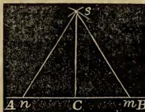
The following is another method, which is preferable, when the given point,  $C$ , is at or near the end of the line.
