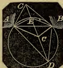
When the bearing of the base line on shore is known, as it generally is, and the bearings to its extremities, or even to one extremity, are taken, the triangle is known at once.
