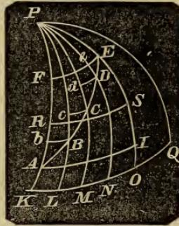
But this departure is neither  $EF$  nor  $AI$ , it is greater than  $EF$  and less than  $AI$ ; because  $bB$  is less than its corresponding portion on  $AI$  and greater than its corresponding portion on  $FE$ . The same may be said of  $cC$ ,  $Dd$ , &c. Therefore the departure on any course corresponds to *neither of the extreme latitudes*, but to *some mean* between the two, and it is so near the arithmetical mean, that the arithmetical mean is taken as the true.
