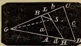
It is necessary to find the area of the triangle  $ABG$ . Conceive a meridian line run through  $B$  ; then we perceive that the angle  $ABG=14^\circ+70^\circ 30'=84^\circ 30'$ . Conceive also a meridian line to be run through  $A$ , and then we perceive that the angle  $BAG=86^\circ 30'-14^\circ=72^\circ 30'$  ; whence  $AGB=23^\circ$ . With the angles and the side  $AB=15.20$ , we readily find  $AG=38.72$ ,  $BG=37.10$ , and the area  $AGB=280.65$  square chains.
