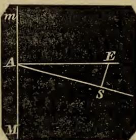
From  $S$  take  $SE$ , of such a value as will make  $SAE 9^{\circ} 17'$ , which is determined by trigonometry ; as follows,
