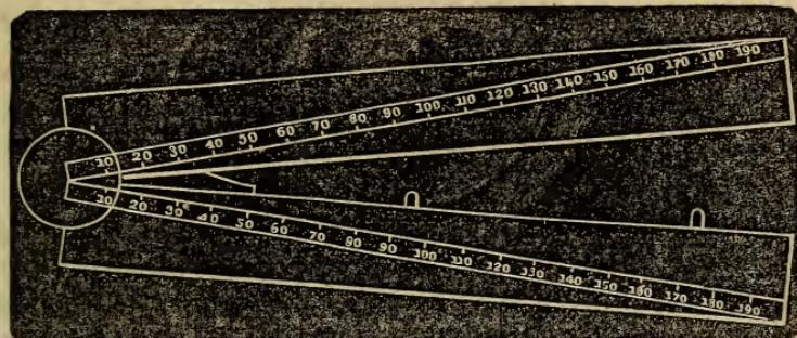
The figure before us represents one side of a sector with the plane scale only upon it. More than one scale can be put on to a side, but we represent but one to avoid confusion.
