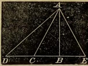
*Demonstration.*—The areas of triangles are as their bases multiplied into their altitudes, but here all the triangles have the same altitude; therefore multiplying the bases into that altitude gives the same proportional product, and the areas of the triangles are as  $m, n, p$ .
