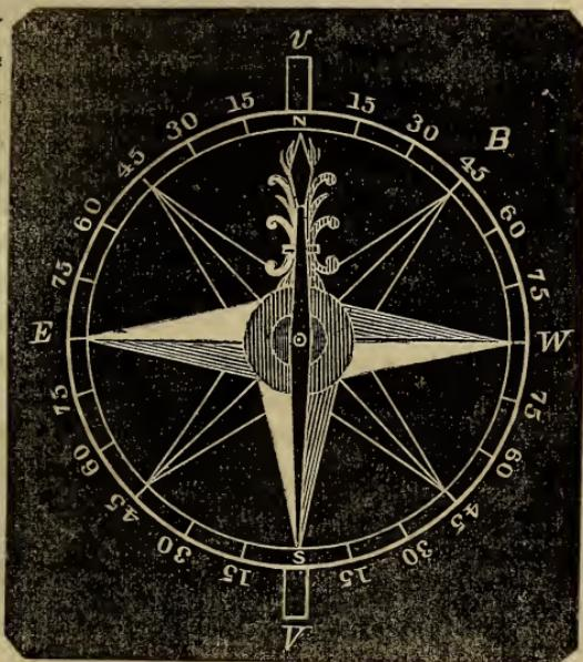
We now *read* the degree pointed out by the north end of the needle, and we find it to be about  $50^{\circ}$  on the arc between  $N$  and  $E$ , showing that the course or direction from the center of the compass to  $B$  is North about  $50^{\circ}$  toward the East—a result obviously true.
