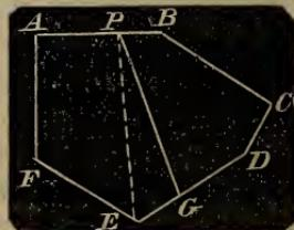
In this figure, let  $PE$  represent such a random line, and let the surveyor compute the area of the figure  $PAFE$ , thus cut off, which area will be *equal to*, or *greater*, or *less* than one of the required parts. We will suppose it *less*; then subtract it from the required portion  $mc$ , and let the triangle  $PEG$  represent that *known difference*, which we shall designate by  $t$ .
