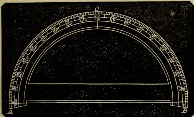
The degrees are numbered both ways, from *A* to *B* and from *B* to *A*. There is a small notch in the middle of *AB*, to indicate the center.
