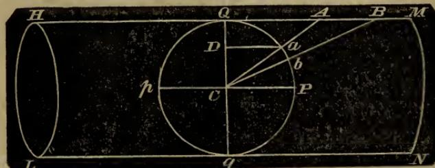
Let  $Qq$  be the plane of the equator,  $Pp$  the earth's axis; conceive a globe enclosed in the cylinder,  $HLNM$ .
