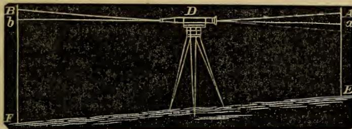
Let *ab* represent the true horizontal line, but suppose that the instrument is so imperfect, or out of adjustment, that when the leveling tube *CD* is horizontal, the telescope would point out the *rising line* *DA*, and the rise would be *Aa*. On turning the instrument round and sighting to *B*, the rise must be the same as in the opposite direction: *for the distance is the same*, therefore *A* and *B* are as truly on a level with each other as *a* and *b*.
