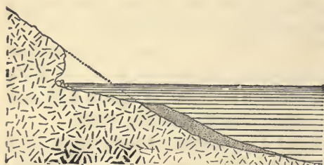
FIG. 43.—SECTION OF A CUT-AND-BUILT TERRACE.
