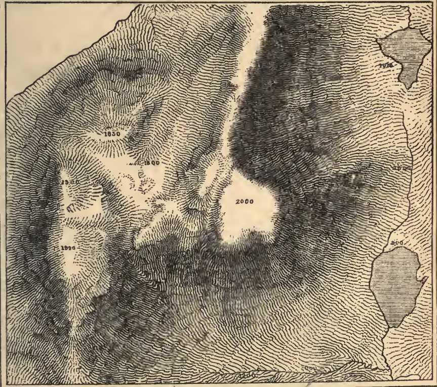
HORIZONTAL AND VERTICAL SYSTEMS OF HILL SHADING (FROME'S SURVEYING).
