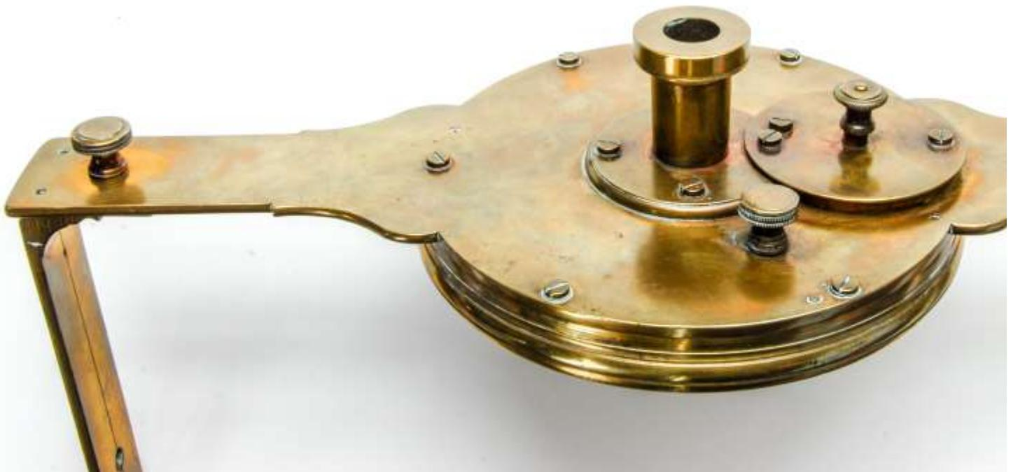
**Surveyor's Compass -- Bottom -- showing mounting post, 2 knobs for counting dials and 2 knobs for mounting the sighting vanes.**
