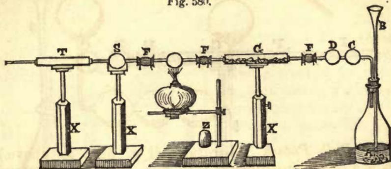
Fig. 580 represents a still more complicated arrangement, in which the product obtained, as in the preceding figure, is subjected to still further operations, by the materials introduced at S or T. A glass spirit-lamp, mounted on a movable arm, and rod attached to a foot, as represented at Z, is a convenient appendage.
