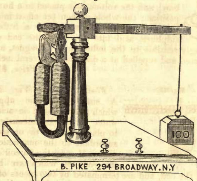
over the poles of the magnet, the coils on the electro-magnet are attached by their ends to the screw cups on the base, or conveniently connecting with the battery.
