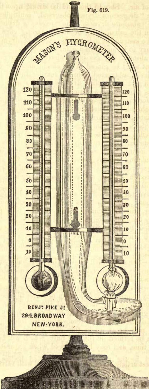
currents of air. Should the wind be strong upon the instrument, the "degrees of dryness observed," multiplied by two, gives the "absolute dryness" (the "excess of dryness" being omitted in the calculation), because a strong current of air makes the instrument indicate the excess of dryness, which is necessary to be added in a calm atmosphere.
