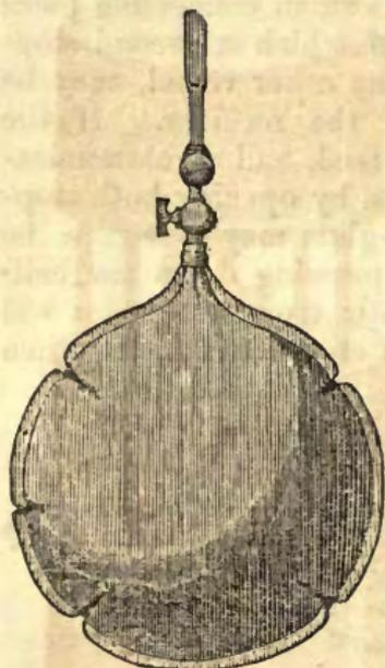
*Flexible Gas Bags.*—(Fig. 527.)—Gas bags made of India rubber cloth are very convenient for holding gases; they are made of various sizes, from one foot to two feet in diameter. One is represented in the cut, having a large stop-cock and mouth-piece, as used for inhaling nitrous oxide gas.
