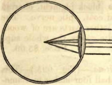
*Model of Double Convex Lens and Rays Converging.* — (Fig. 692.)—The focal distance, or distance of the focus from the surface of the lens, depends both upon the form of the lens and of the refractive power of the substance of which it is made; in a glass lens, both sides of which are equally convex, the focus is
