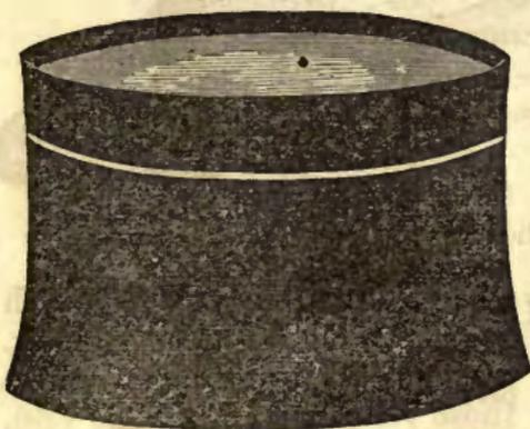
*Engraver's Magnifier.*—(Fig. 664.)—The engraver's magnifier consists of a convex lens, about one and a half inches in diameter and two inches focus, set in a deep horn case, which is usually supported over the work to be engraved by a suitable stand; the eye viewing the work through the lens while engraving.
