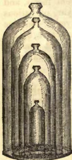
*Bell Glass Receiver.*—This is used in experiments on the air, or gases, and is a glass vessel of the shape represented in Fig. 481, and of various sizes, from a gill to several gallons. There is a knob on the top, which is used as a handle for moving it by.
