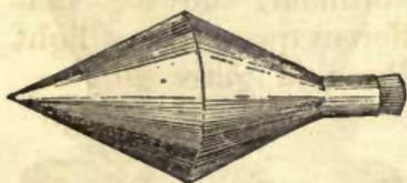
*Hydrogen Gas Generator.*—(Fig. 539.)—This represents nearly the same apparatus as the last, of a larger construction, producing and containing a greater quantity of gas, and particularly useful in chemical experiments where a supply of hydrogen is required. On the top of the plate there is a stop-cock of the usual size of the cocks in chemical apparatus, having a brass jet for burning the gas. Price, \$4.00 and \$6.00.
