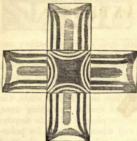
If two unannealed rectangular pieces of glass are crossed at right angles the structure of the fringes will be varied in a similar manner to those represented in the drawing annexed.
