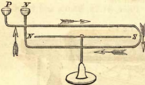
*Apparatus for Oersted's Experiment.* —
