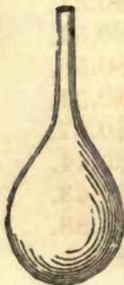
*Flasks.*—(Fig. 482.)—These are made of glass, They are used in distilling and boiling various solutions, and will stand a greater heat without breaking than any other description of glass.
