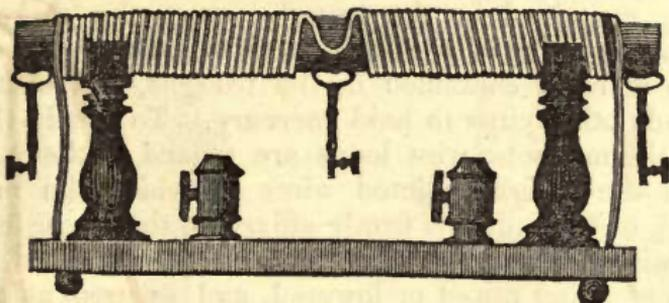
instrument. On passing the battery current through the coil, the ends become similar poles, and the middle an opposite pole. And by changing the direction of the current the poles will be reversed.
