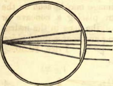
*Model of Plano-Convex Lens and Rays Converging.* — (Fig. 693.)—Lenses that have one side flat and the other convex, are called plano-convex, and their focus is at the distance of the diameter of a sphere, of which the convex surface of the lens forms a portion, as represented
