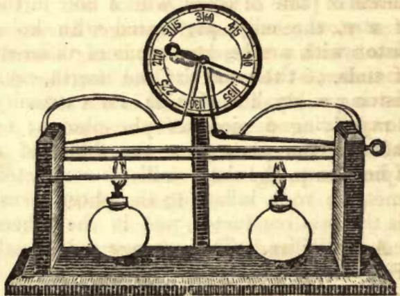
*Pyrometer.*—(Fig. 555, as above.)—This arrangement consists of a base of mahogany about twelve inches long, to which are attached two upright pieces which are immovably held in their position by metallic braces, extending from the one to the other; between these there is a rod of metal, supported at one end from the point of a screw, and at the other from the shorter end of a bent lever, the axis of which is fastened to the wood. The longer end of the lever
