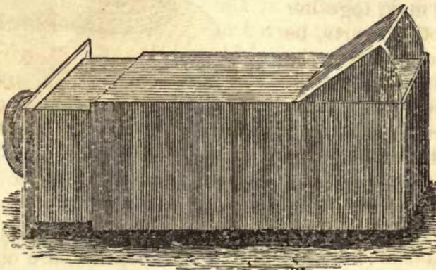
*Directions for Use.*—Place on the ground glass a piece of good tracing paper, and present the instrument to the object to be copied, which should be strongly illuminated. The camera should be placed level. Draw the slide till the object is reflected on the paper, and if the lines are followed with a pencil, a correct copy of the view will be obtained. If a portrait be desired, the person should be placed in the
