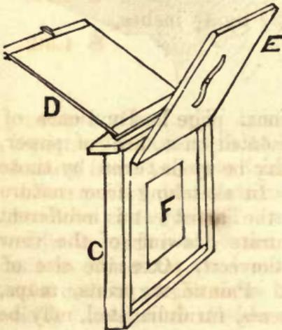
B, may be withdrawn, and another frame, C (represented in Fig. 705), introduced, consisting of a box, made to receive thin wooden frames, which are grooved around and adapted for receiving the various sized daguerreotype plates to be used. This frame is furnished with a sliding shutter, D, in front of the plate to prevent the access of light to the plate till placed in the camera. E is a hinged flap with spring to keep the frame and plate in their proper position.
