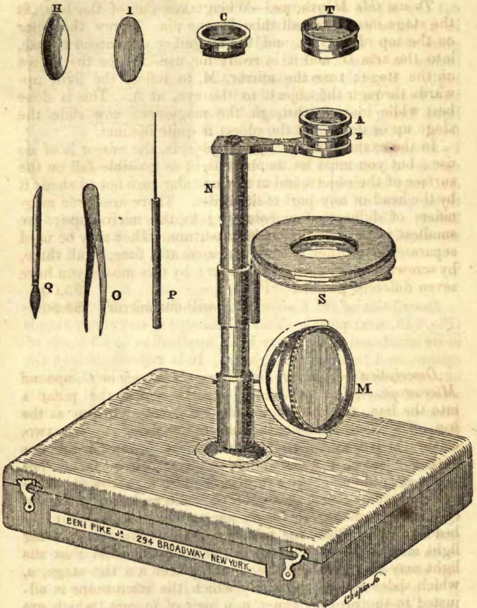
The magnifying powers in this microscope are as follow : No. 1, 36 times ; No. 2, 64 ; No. 3, 100 ; Nos. 1 and 2 combined, 169 ; Nos. 1 and 3, 256 ; Nos. 2 and 3, 400 . Nos. 1, 2, and 3, 676—superficial measure.
