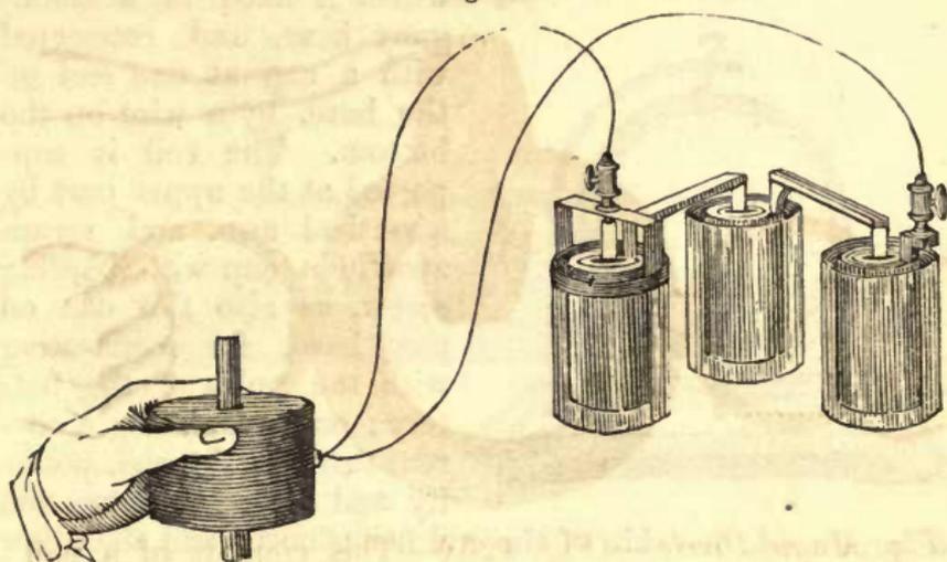
The battery required to perform this experiment with advantage should be of a power not less than three of "Grove's series," of the usual size.
