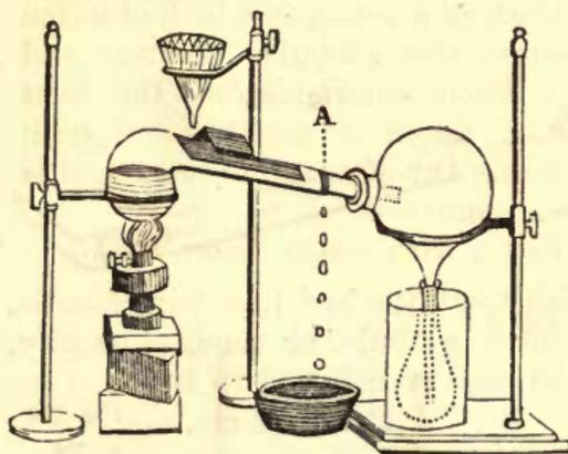
*Apparatus for Distillation and Condensation of Liquids.*—(Fig. 570.)
