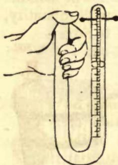
*Ure's Eudiometer* (Fig. 565) consists of a glass tube bent in a U form and closed at one end, the closed tube being graduated into 100 equal parts, and having inserted near the end, two platina wires, the outer extremities being formed into rings, or small balls for the passage of an electric spark.
