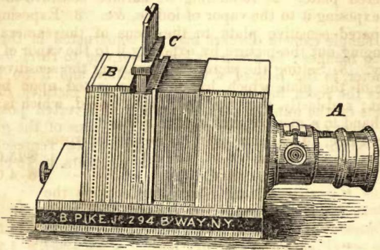
*Daguerreotype Camera.*—The camera obscura, used for taking daguerreotype pictures (Fig. 704), consists of a mahogany box, on the front of which is fixed a brass sliding tube, A, containing two achromatic lenses. The image is received on a piece of ground glass, fitted in a frame, B, which slides in a groove in the back of the camera, and the focus is adjusted to the greatest nicety by a fine rack-work movement in the brass tube containing the lenses. The frame,
