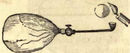
The above cut (Fig. 526) represents a brass tobacco-pipe, furnished with a stop-cock, that it may be connected with a bladder for throwing up soap-bubbles, filled with hydrogen gas, or with a mixture of hydrogen and oxygen gas, for explosion. Blow some soap bubbles, filling them from the bladder of hydrogen, furnished with a brass pipe; they will ascend rapidly to the ceiling; if they are intercepted in their course by a lighted candle, they will explode with a dull
