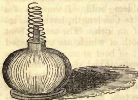
*Flameless Lamp.*—(Fig. 546.)—The aphlogistic, or flameless lamp, having a glass instead of metal tube for supporting the wick; a fine platinum wire about fifteen inches long, and wound in the form of a spiral spring, is placed partly over the end of the wick. The lamp thus pre-
