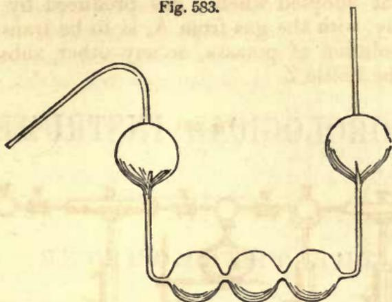
*Five Bulb Potash Apparatus.*—(Fig. 583, as above.)—This is a glass instrument with five bulbs, for containing solution of potash to absorb the carbonic acid produced in an analysis, made very light, of the shape of the cut, and also after Liebig's pattern. Price, \$1.25.
