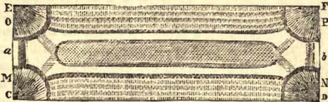
in the bent state, double refracting properties. Two sets of colored fringes are perceived, one on the convex or dilated side of the plate, and the other on the concave or compressed side. Between these two sets of fringes is a black line, indicating the situation where neither compression nor dilation exists, and where, therefore, double refraction is absent.
