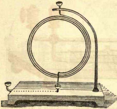
which is fixed in a mahogany base, and connected with a cap at one end of the base, by a wire on the bottom. The coil is supported at the upper part by a vertical arm, and terminates in a cup with binding screw, as also the one on the base, for connecting with the poles of the battery; on transmitting a current through the coil, polarity and magnetic attraction
