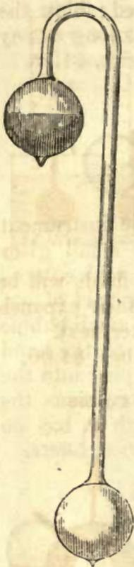
main filled with steam. The open bulb is then closed, by melting the glass at its capillary termination. When the empty bulb is immersed in a mixture of salt and snow, the vapor existing within it is condensed, which removing pressure from the surface of the water in the other bulb, enables it to evaporate rapidly; and the vapor being condensed as speedily as it is formed, the water is readily frozen.
