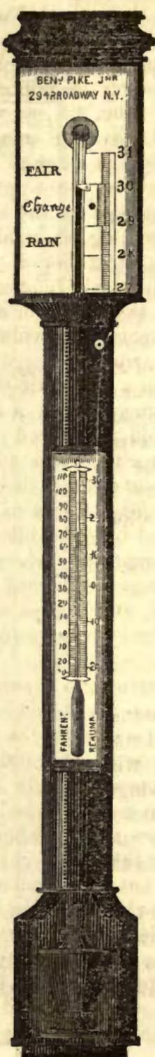
*Best flat front Barometer.*—(Fig. 606.)—The best flat front mahogany case barometer having vernier and glass door, with large thermometer in the body of the case, having a long cylindrical bulb to the tube, exposing thereby a large surface to the atmosphere, graduated to Fahrenheit and centigrade scales, and covered with glass, portable screw at the bottom, and the case highly polished. Price, \$16.00.
