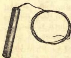
A pair of brass conductors (Fig. 475.) for the hands, being the most convenient form for applying the fluid to the system for general purposes. These accompany the best magnetic instruments.
