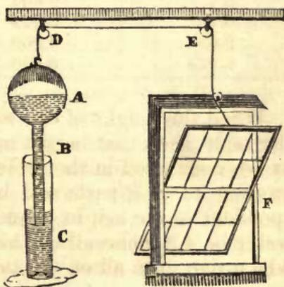
with mercury, and in this state is inverted, and the end plunged in a jar of the same fluid; to the top of the ball is attached a string, which, after passing over the pulleys, D and E, is finally fastened to the window, F. When the heat of the apartment rarifies the air in the ball, the mercury is driven out, and the ball and tube being thereby lightened, rise and suffer the window to swing itself open. An increase of cold will produce the contrary effect.
