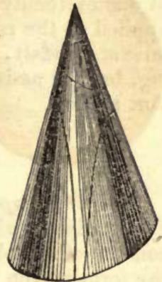
*Dissected Cone.*—(Fig. 774.)—The dissected cone is used for illustrating the conic sections. It is formed of a cone of hard wood cut in parts representing these sections, as the ellipse, parabola, hyperbola, which may be put together by short pins in the parts forming the complete cone.
