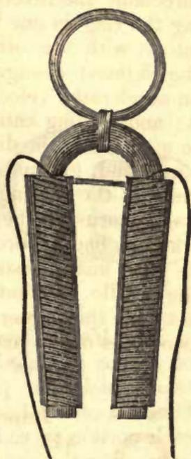
*Large Electro-Magnet.*—(Fig. 425.)— This cut represents one of the most elegant modes of mounting large electro-magnets. The magnet is mounted, poles upward, on a firm and substantial base, having a pillar with an arm, or lever, passing through a mortice on the top of it; the lever being attached to the lifter
