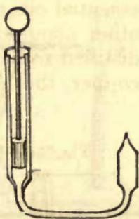
*Glass Syringe.*—(Fig. 567.)—This instrument is formed of a piece of straight glass tube drawn at one end to a point, having a piston packed with tow attached to a wire handle. By means of this instrument a globule, or small quantity, may be drawn into the tube, and transferred to any other vessel.
