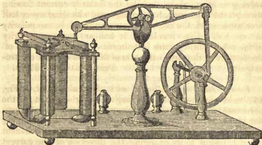
*Magnetic Beam Engine.*—(Fig. 452, as above.)—This cut represents a small working model of an electro-magnet motive engine, on a stout mahogany base five inches wide and
