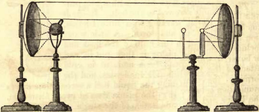
*Reflectors, &c., for Radiation of Heat.*—(Fig. 562.)—Reflectors arranged for the radiation of heat, commonly called *Pictet's Apparatus*, consist of two concave reflectors, or mirrors of brass, or planished tin, twelve inches or more in diameter, and mounted on mahogany stands, having rods,
