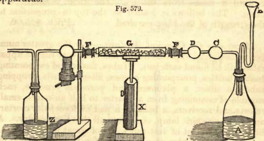
In Fig. 579, the gas is made to act upon I. The assay is often placed in tubes, as G. This figure illustrates the
