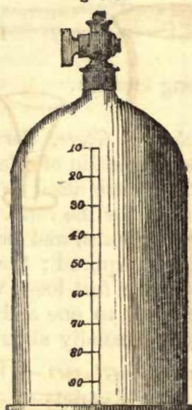
*Graduated Measure Glasses.*—(Fig. 495, as above.)—These are made of strong glass, and are used for measuring liquids. They are of various sizes, but one of six ounces is the most useful. The quantity is marked by a graduated scale at the side, and usually commences with half a drachm, and so proceeds drachm by drachm to half an ounce, and upwards to an ounce or more.
