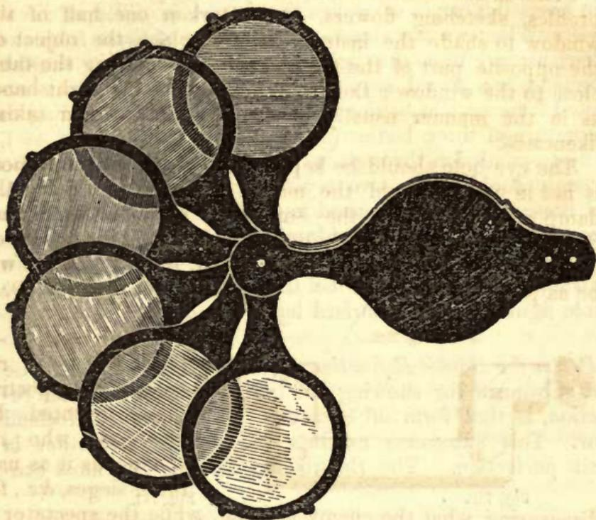
*Claude Lorraine Glass.*—(Fig. 709.)—This consists of a variety of different colored glasses, about one inch in diameter, mounted in horn frame and turning on one centre, for producing a great variety of colors and showing their combination; it also will be found both pleasing and useful for viewing eclipses, clouds, landscapes, &c.
