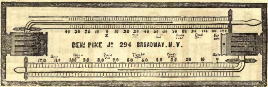
*Self-Registering Thermometer for extreme Heat and Cold.*
