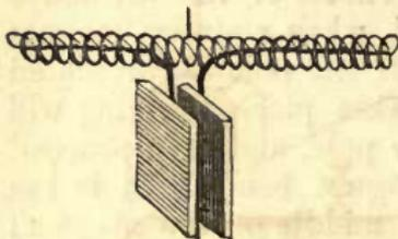
*Floating Coil.*—(Fig. 423.)—A simple galvanic apparatus, which when placed in acidulated water turns spontaneously, so as to place itself north or south, or accordant to the magnetic meridian. It consists of a coil of wire, the ends of which are brought
