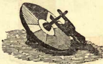
rapidly spun around for a considerable time. On the surface of the top there is accurately described the proportion of the different colors, which are engraved on a plate, near the centre, while the exterior is filled with colored papers, each color of nearly the color of the spectrum, and occupying the same proportion, viz. violet 80, indigo 40, blue 60, green 60, yellow 48, orange 27, red 45; the whole is varnished to protect it from injury.
