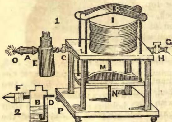
*Gurney's Oxyhydrogen Blow-pipe.*—(Fig. 537.)—A compact, powerful, and perfectly safe, instrument, for procuring a constant and intensely powerful flame, applicable to the usual purposes of a blow-pipe; that is, the melting of small quantities of refrac-
