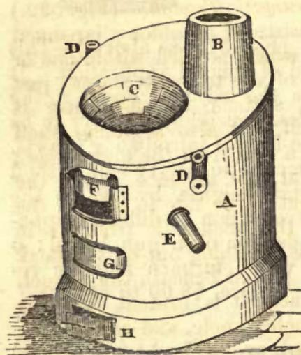
*Dr. Black's Furnace.*—(Fig. 520.)—A very serviceable portable furnace; used for chemical operations, and which may be applied to numerous other purposes.
