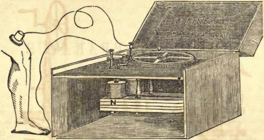
a cog-wheel on the spindle, acting in the teeth of a larger wheel, which is turned by the hand, thus preventing the trouble of constantly adjusting the bands, as in the usual construction; the whole is enclosed in a mahogany case, and may either be used in the box, or taken out.
