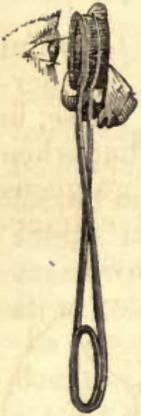
*Tourmaline Polariscope.* — (Fig. 712.)— Two plates of tourmaline are mounted in cells capable of being rotated on their axes, and supported before each other by a spring frame, between which crystals may be conveniently supported, and the system of beautiful rings observed, represented in Fig. 713, 714, 715, and 716.
