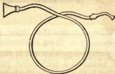
though, for the sake of portability it is often curved; they are also recommended of a parabolic figure having the apex of the paraboloid cut off, and the mouth of a small tube inserted in the focus, to convey the sound concentrated at that point to the auditory organ. Various other forms are adopted in practice; and of late, flexible India rubber tubes formed over a spiral wire (Fig. 780) have been brought into
