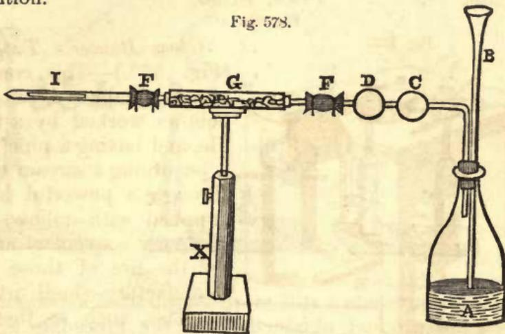
(Fig. 578, as above), A, represents bottles, flasks, or retorts, for producing the gas required; B, a long funnel for introducing acid in small successive quantities, or any other liquid that may be required; C D, balls for intercepting any portion of fluid which may be mechanically suspended in the gas escaping from the bottle; G, the tube filled with fragments of chloride of calcium for drying the gas; F, caoutchouc connectors; X, wooden stands for supporting the apparatus.
