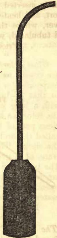
*Iron Retort for Oxygen.*—(Fig. 487, as above.)—This is an iron vessel shaped usually in the form of a bottle, holding from one pint and upwards, and having an iron tube, bent or straight, screwed, or ground conically into the neck, and is used principally in producing oxygen gas.
