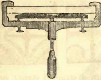
*Polarization by bending a Glass Tube.*—(Figs. 726 and 727.)—Analagous effects are produced by slightly bending a piece of annealed glass in a suitable frame. To illustrate this, a slip of glass about six inches long, half an inch wide, and one-third of an inch thick, is confined in a suitable brass frame,
