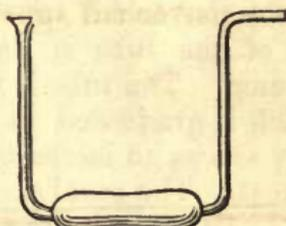
*Drying Tubes.*—(Figs. 584 and 585, as above.)—Bent tubes in which organic bodies are dried, used in organic analysis. Price, 37 to 75cts.
