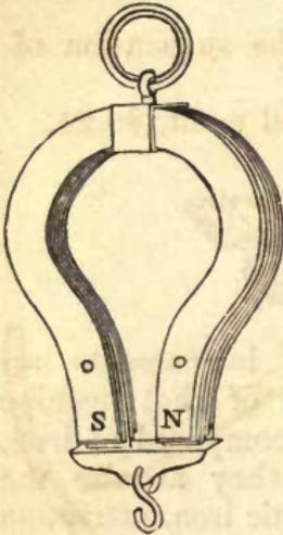
*Compound Horse-shoe Magnet.*—(Fig. 411.)—Compound horse-shoe magnet, or battery of single horse-shoe magnets, held together by screws or other contrivances. The association of several bars is a set. Mounting with an appropriate armature greatly increases the magnetic power, not only for suspending weights, but also the capability of making other magnets.
