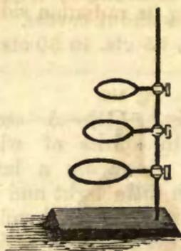
Retort stands with rectangular iron base, ten inches long, having two rods and six rings of the size of the former.
