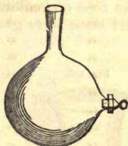
*Globe Receivers.*—(Figs. 488 and 489, as above.)—Receivers are vessels, usually of glass, of a spherical form, with a straight neck, into which the neck of the retort is usually inserted. When any proper substance is put into a retort, and heated, its volatile parts pass over into the receiver, where they are condensed. They are made plain and tubulated, with ground stoppers.
