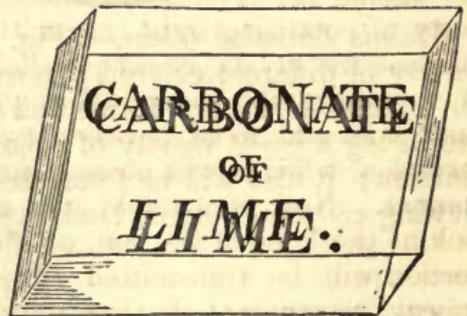
venient. Let a black line be drawn on a piece of paper, and let a rhomb of this spar be laid upon it; then, on look-through the upper face of the spar, down on the paper, two lines will be seen, and any object viewed at a distance
