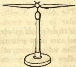
*Magnetic Needles.*—(Figs. 412 and 413, as above.)—Magnetic steel needles of various lengths and forms, mounted with central hard metal caps for suspending on pointed stands, for the purpose of illustrating the influence of terrestrial magnetism as regards the horizontal directive force: also the polarity of a magnetic body, by its attractive and repulsive qualities, in relation to similar and dissimilar poles.
