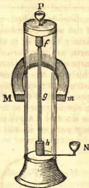
When the circuit is completed through the gold leaf, the latter will be attracted or repelled laterally by the poles of the magnet, according as the current is ascending or descending; the
