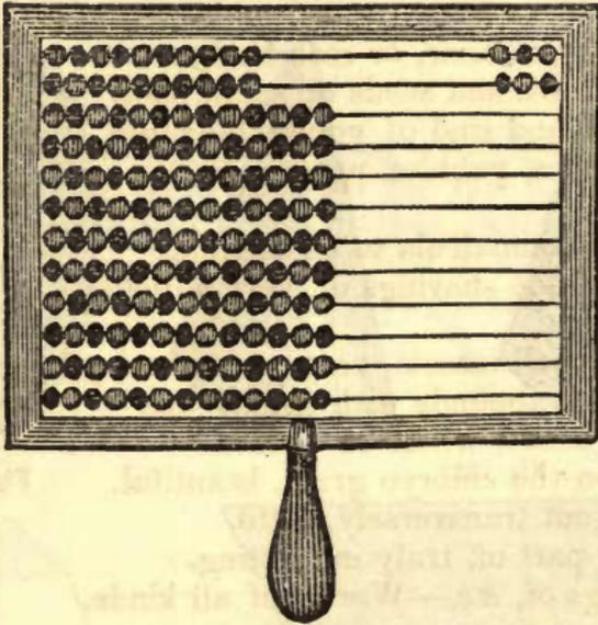
*Numeral Frame* (Fig. 761) consists of a strong frame with a handle, having twelve wires passing through the frame, on each of which are twelve balls, a black and a yellow one alternately; designed to give children a distinct idea of numbers and their combination.
