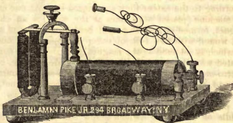
*Magnetic Machine Vibrating from both Poles.*—(Fig. 470, as above.)—This instrument is the same as the preceding one, but the armature vibrating from both poles of the magnet; the spring being supported by a brass pillar fixed on one of the brass bands that secure the helix to the board. This instrument vibrates with great force, but the former instrument is the least liable to derangement. The wires
