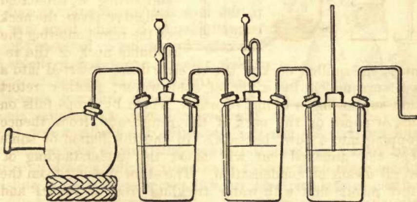
*Woolf's Apparatus.*—(Fig. 572, as above.)—The most elegant and convenient method of impregnating water with an absorbable gas is by means of Woolf's apparatus, which
