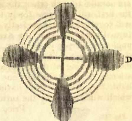
*Selenite Designs.*—Numerous splendid and beautiful effects are produced by arranging plates of selenite of different thicknesses and designs, on plates of glass. These, in ordinary light, will appear perfectly transparent; but when viewed in polarized light, will exhibit the most gorgeous coloring, and may be made to undergo the most extraor-
