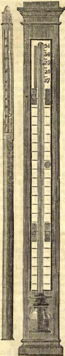
the higher we ascend the rarer it becomes. At 31 inches a fall of one-tenth of an inch indicates a height of 82 feet; at 30 inches, 85 feet; at 29 inches, 87 feet; at 28 inches, 91 feet; at 27 inches, 94 feet; and at 26 inches, 98 feet; for every tenth of an inch the mercury falls.
