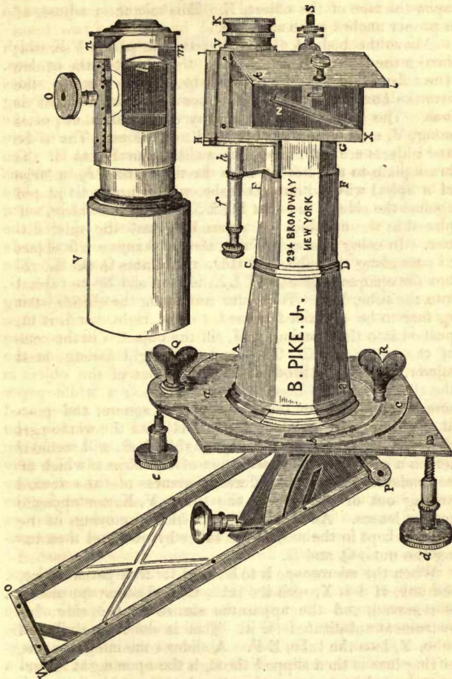
the opaque object, it is received by a mirror, M, placed in the box, H I L X, which reflects the condensed light back upon the face of the object, E. This mirror is adjusted to a proper angle by the screw, S.
