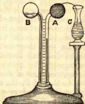
it to the covered ball. This acts as a syphon, and keeps the ball moist. The graduated scale shows the degree of evaporation. When this hygrometer stands at  $15^{\circ}$ , the air feels damp, from  $30$  to  $40^{\circ}$  we reckon it dry, from  $50$  to  $60^{\circ}$  very dry, and from  $60^{\circ}$  upwards we should call it intensely dry.
