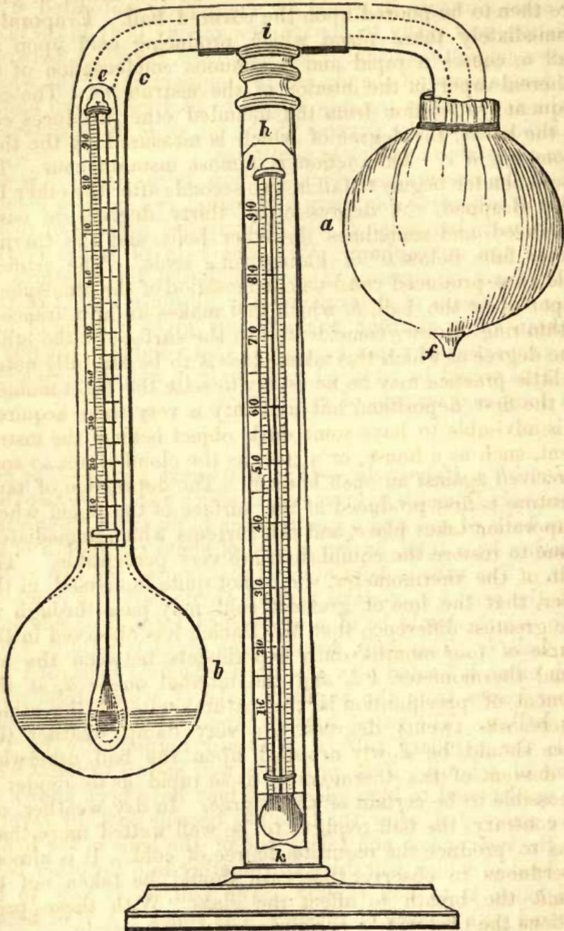
The manner of using the instrument is this:—After having driven all the ether into the ball *b*, by the heat of the hand, it is to be placed in an open window, or out of doors, with the ball *b* so situated as that the surface of the liquid
