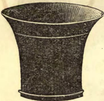
*Watchmaker's Magnifier.*—(Fig. 663.)—The watch magnifier consists of a convex lens of about two inches focus, set in a deep horn case, the larger end of which is of such a size and form, as to be held between the eyebrow and bone of the cheek without inconvenience. The cut represents the size of the article.
