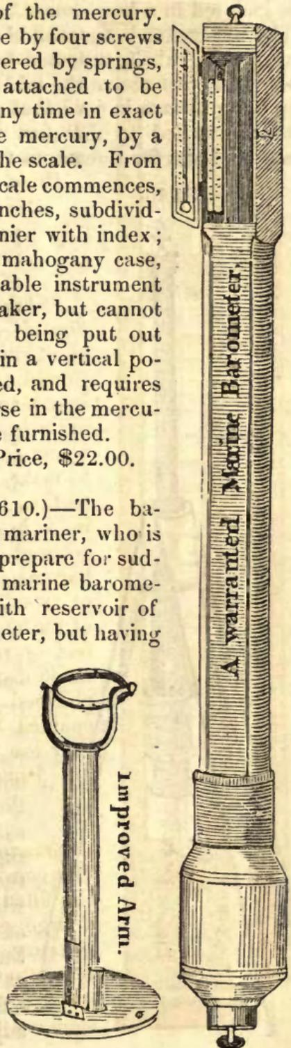
inner side of which is fixed a thermometer. The reservoir is inclosed in a brass case, having a portable screw beneath. The barometer is suspended in a vertical position, by a brass arm and gimbals, attached by thumb-screws to the side of the case, just above the middle, which allows the barometer to hang always in a vertical position, however the ship may roll; attached to the arm there is a stout circular plate, having holes for screws, to fasten the instrument to any part
