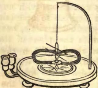
The compass, wire, and card, are enclosed in glass in order to secure them from the agitations of the air, and to allow of our seeing the position of the needle.
