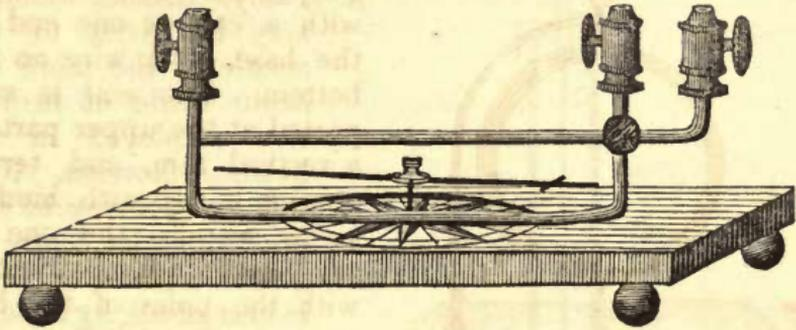
(Fig. 431, as above.)—This cut represents the same instrument, mounted on a mahogany base, having a graduated circle for estimating the deviations of the needle.
