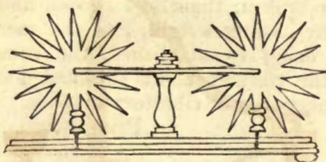
This instrument is also constructed with two wheels, as represented in Fig. 440. An electro-magnet is sometimes substituted for the steel magnet, being included in the circuit with the wheel,
