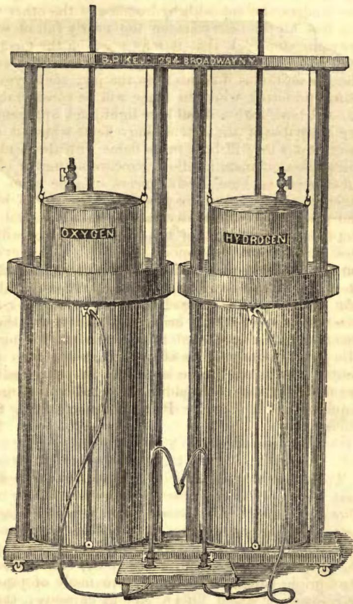
*Compound Blow-pipe and Pneumatic Cistern.*—(Fig. 536, next page.)—The compound blow-pipe with pneumatic cistern combined, consists of a stout oblong cistern having two gas holders in the form of square boxes; the one for hydrogen being the largest. The gas holders are confined in their places by being slid under projections on the sides of the cistern, so that they cannot rise when filled with gas, and
