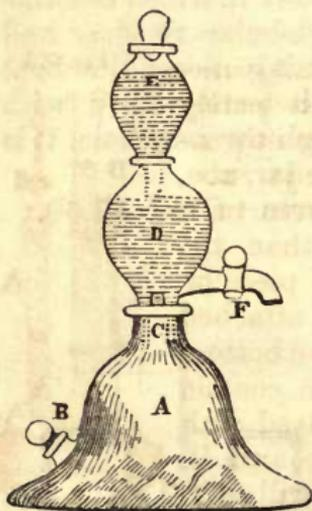
*Nooth's Apparatus.*—(Fig. 573.)—There are various kinds of apparatus for impregnating water with carbonic acid. One of the most elegant and simple is Dr. Nooth's, represented in the cut.
