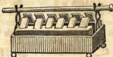
*Cooper's Lamp Furnace.*—(Fig. 516, as above.)—A lamp which is made of an elongated form, and is furnished with two rows of broad wicks, the whole or part of which may be lighted at once. Professor Faraday recommends this simple furnace as valuable for the heating of tubes, or any long and narrow vessel. Near the ends are two twisted wires, for the support of the tube to be heated.
