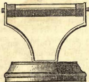
*The Prism.*— (Fig. 698.)—A triangular piece of glass employed to separate a ray of light into its constituent parts or colors by refraction. The prism is the instrument by which the most remarkable phenomena of light and colors are exhibited. To use the prism, let a room be darkened, and the sun permitted to shine into it through a small hole in the window shutter,
