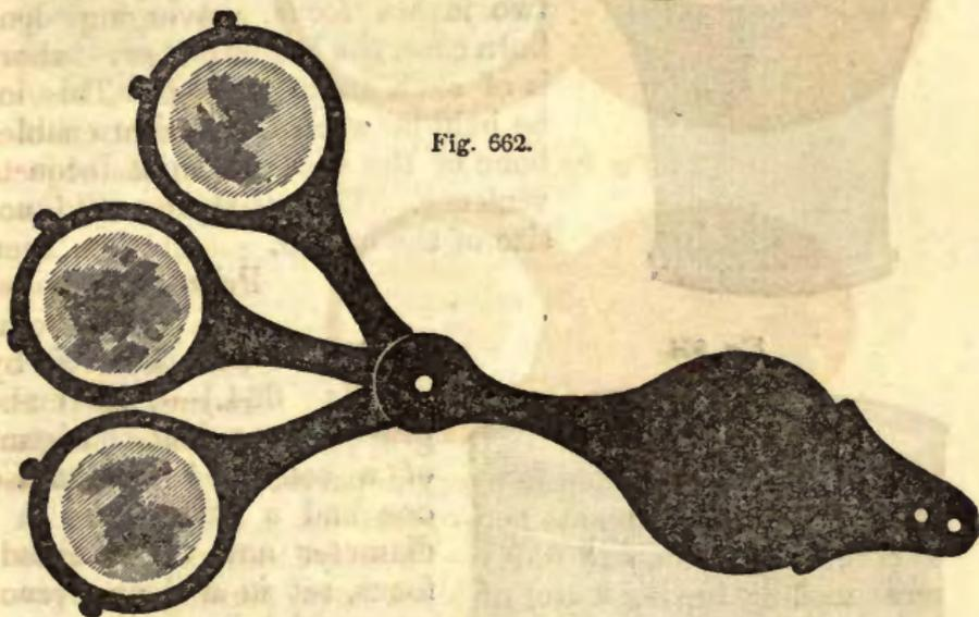
*Botanical Lenses, or Magnifiers.*—The haste with which botanists, &c., frequently have occasion to view objects, renders a pocket magnifier very useful. The most convenient of any constructed are those represented in Figs. 660, 661, and 662, which are drawn of the medium size, there being a size smaller and one larger; this form of mounting
