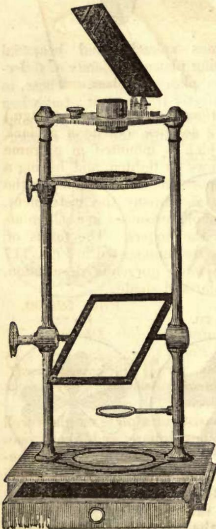
*Biot's Reflecting Polariscope.*—(Fig. 723.)—Biot's reflecting polariscope, as represented in the cut, having polarizing and analysing plates with horizontal movement, and graduated circle; movable stage for crystalline plates, tourmaline cell, double image or Nichol's prism, plane mirror, and condensing lens. The framework of highly finished brass mounted on a mahogany base, with drawer for holding the smaller parts.
