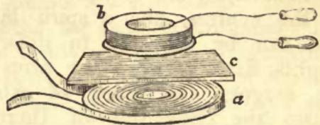
*Flat Wire Coils.*—(Fig. 467, as above.)—These consist of fine insulated copper wire, from 1000 feet and upwards long, wound in the form of a flat spiral, and carefully ce-
