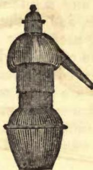
*The Alembic, for Sublimation and Distillation.*—(Figs. 490 and 491, as above.)—The alembic is used for distillation, when the products are too volatile to admit of the use of the retort. The alembic consists of a body, to which is adapted a head. The head is of a conical figure, and has its external circumference or base depressed lower than its neck, so that the vapors which rise, and are condensed against its sides, run down into the circular channel formed
