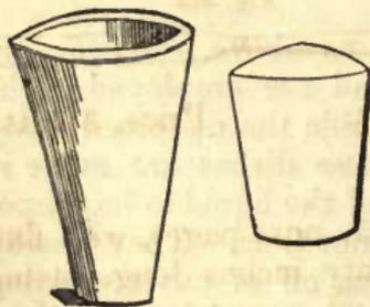
*Crucibles.*—(Fig. 509.)—The crucible is a vessel usually made of well hardened earthen or stone ware, in constant use in the chemical laboratory for performing fusions of metals and other substances.
