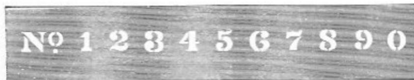
It is desirable to have drawings plainly and uniformly lettered and numbered, and to do this easily and rapidly, a transparent stencil, as shown above, may be used to advantage, either with the brush or by first outlining the figures with a sharp pointed pencil, and afterwards inking them with a pen.
