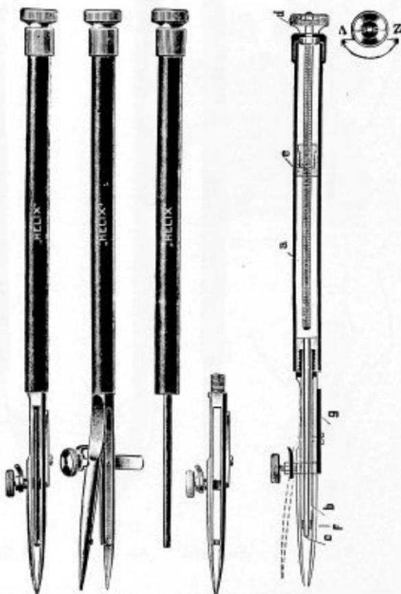
This Ruling Pen is constructed so as to overcome each and every inconvenience during its use. No drying of the ink. No soiling of the Pen, the Set-square nor of the fingers; always ready for use. Very easily filled by a small turn to the right side of the screw and a sufficient quantity of ink is drawn into the piston rod. A great deal of time saved.
