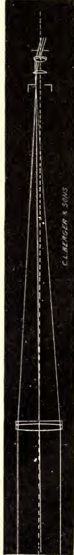
Cross section of the Berger Engineer's Transit Telescope with inverted image. Diagram shows the path of a pencil of rays in this telescope.
