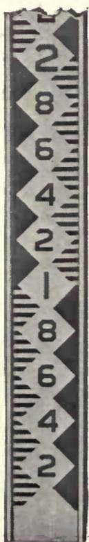
stadia rod. It is twelve feet long and is graduated on a surface two inches wide to feet, tenths and hundredths. The two joints are secured and released by spring catches. The rod being in three sections is carried in a canvas case about three and three tenths feet long.
