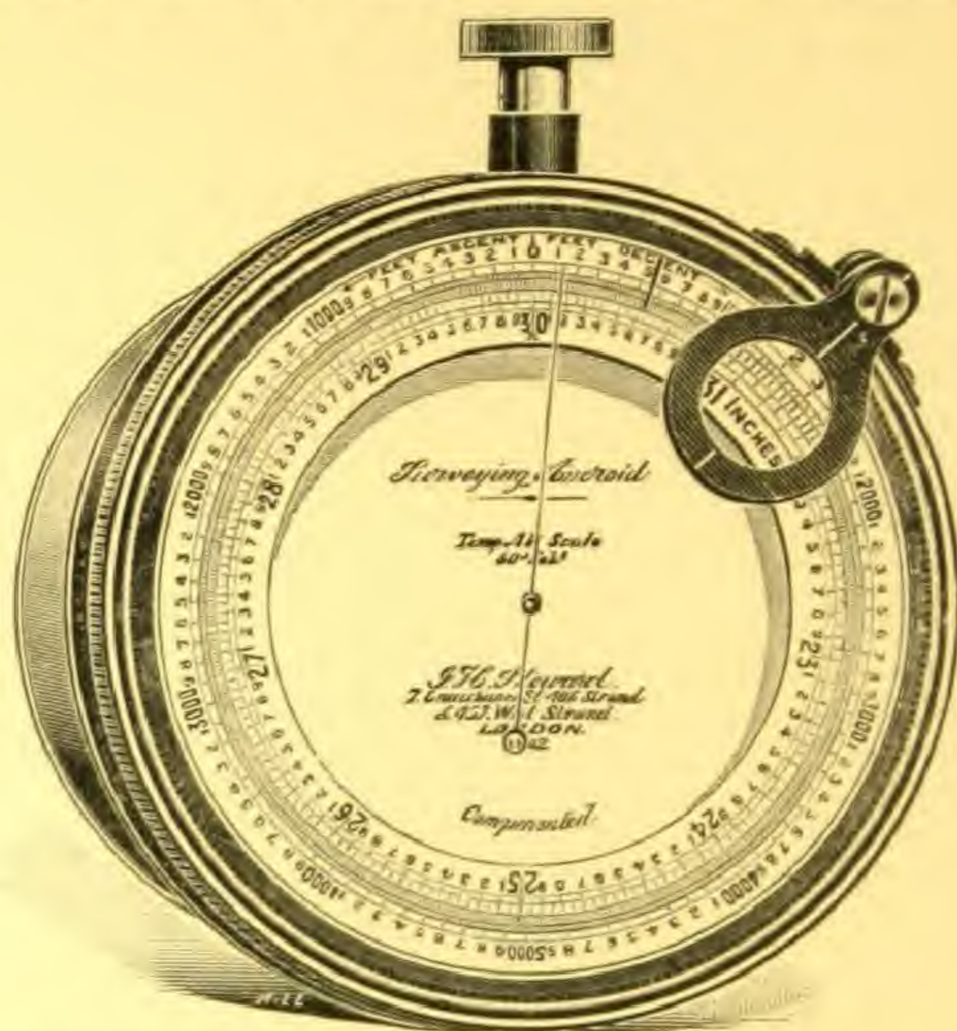
Fig. 109. The Hypsometric Aneroid, with altitude scale to 10,000 feet.
