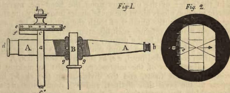
The divisions on the graduated circle indicate spaces of five minutes each, which are read off along with the *degree*, by means of an index-pointer. The remaining minutes and seconds, if any, are determined by the reading microscope, as was stated when describing the construction of the circle; it now remains
