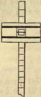
When both the staves are used, they should be set up at equal distances on each side of the spirit-level: the difference of the heights of their vanes will be the absolute difference of level between the two stations. But when one staff only is employed, the difference between the height of the vane and the height of the centre of the telescope of the instrument, will be the apparent difference of level, which, if the distance between the staff and instru-
