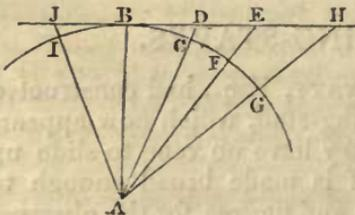
“ But the line of sight, B, D, E, &c., given by the operation of levels, called the apparent line of level, is a tangent, or a right line perpendicular to the semi-diameter of the earth at the point of contact, B, rising always higher above the true line of level, the further the distance is. Thus, C D is the height of the apparent level above the true level, at the distance B C or B D;
