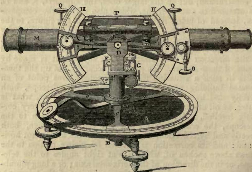
The horizontal circle (or limb), A, of this instrument consists of one plate only, which, as usual, is graduated at its circum-
