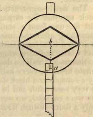
In levelling, the vane must be moved up or down, until the horizontal wire of the telescope bisects the acute angles of the lozenge, or in other words passes through its horizontal extremities, as shown in the figure.
