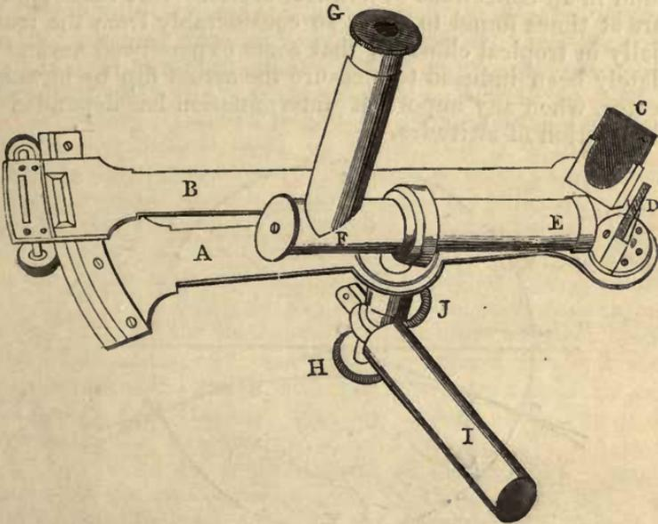
The preceding figure represents this instrument: A is the sector, B the index, with its clamp and tangent-screw, exactly similar to that of the sextant: the index-glass, C, and the horizon-glass, D, are fixed at right angles to the plane of the instrument. The telescope, E F, is fitted into a collar, having an up-and-down motion given to it by turning the screw H; the
