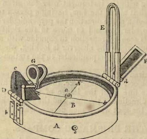
be inclined at any angle, by means of its joint, *d*; and it will remain stationary on any part of the vane, by the friction of its slides. Its use is to reflect the image of an object to the eye of the observer when the object is much above or below the horizontal plane. When the instrument is employed in observing the azimuth of the sun, a dark glass must be interposed; and
