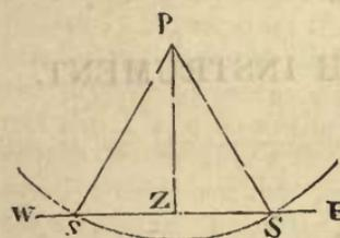
In the accompanying figure, P is the pole, Z the zenith, E Z W the prime vertical passing through the east and west points, the dotted line S s the path of the star; all seen as projected on the horizon from a point above Z. Then in the right-angled spherical triangle, P Z S, P S is the north polar distance of the star, P Z the co-latitude, and the angle Z P S, half the time elapsed from S to s, therefore,  $\tan. P Z = \tan. P S \times \cos. Z P S$ .
