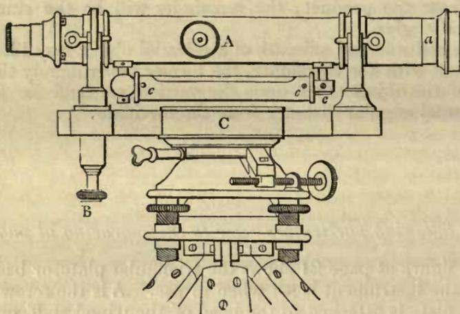
The above figure represents this instrument; it has an achromatic telescope, mounted in Y's like those of the theodolite, and is furnished with a similar system of cross wires for determining the axis of the tube, or line of collimation. By turning the milled-headed screw, A, on the side of the telescope, the internal tube, *a*, will be thrust outwards, which carrying the object-glass, it is by this means adjusted to its focal distance, so as to show a distant object distinctly.
