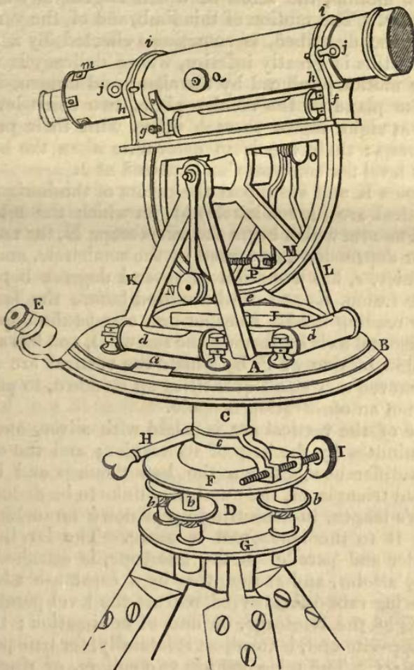
Beneath the parallel plates is a female screw adapted to the staff head, which is connected by brass joints to three mahogany legs, so constructed that when shut up they form one round staff, secured in that form for carriage by rings put on them; and when opened out, they make a very firm stand, be the ground ever so uneven.
