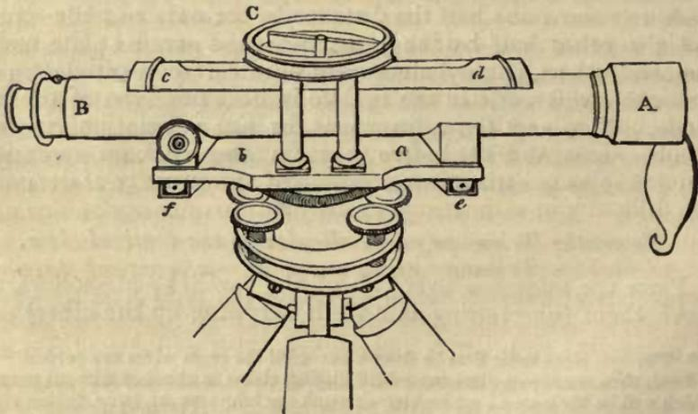
The telescope, A B, rests upon the horizontal bar, *a b*, which turns upon the staff-head (similar to the one employed in the
