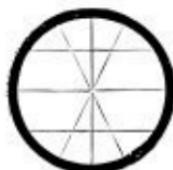
Diaphragm showing arrangement of wires as used with our mine transits, to distinguish center horizontal wire from stadia wires, to avoid mistakes.
