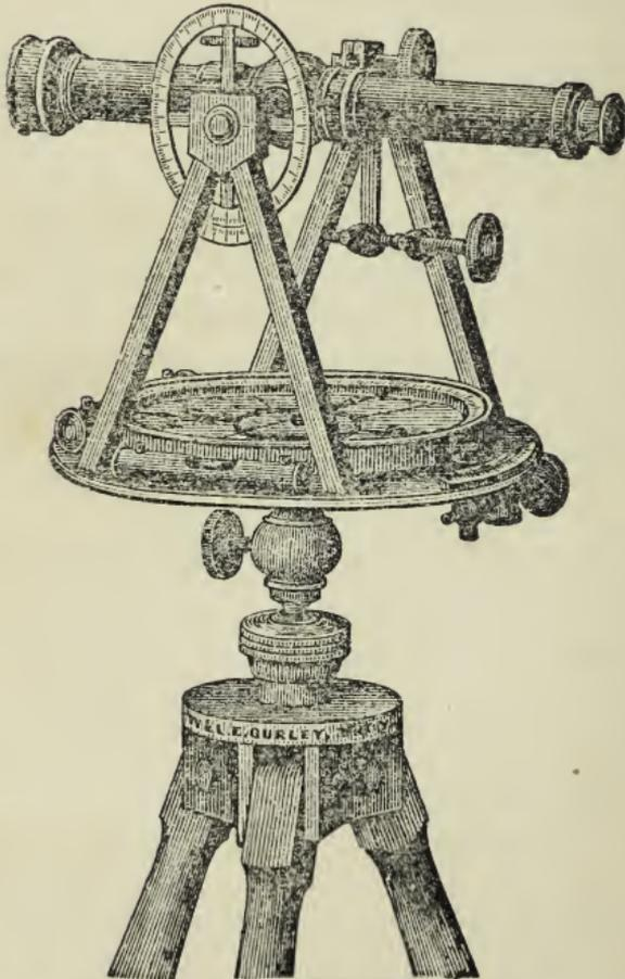
The Vernier Transit, or Transit Compass, represented in the cut above, has the same general properties as the Vernier Compass, but is furnished with a telescope in place of the ordinary sights.
