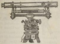
Of a superior quality, with long Bell Metal Centres, Detached Parallel Plates, to pack in the Case, thereby securing the safety of the Tangent Screws, &c., in transport-
