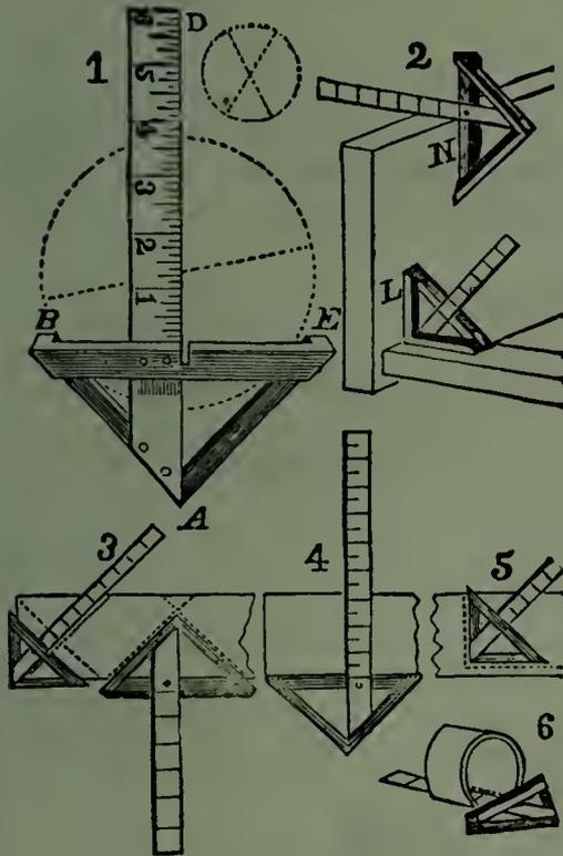
This square combines, in a most convenient form, *five different instruments*, viz., The TRY-SQUARE, the MITER, the T-SQUARE, the GRADUATED RULE, and (what is entirely new) the CENTRE-SQUARE, for finding the centre of a circle.
