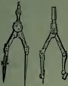
There are two kinds of bow pens and bow pencils. Those represented by Nos. 84 and 85 are about three inches long, and the legs are extended and closed by the pressure of the fingers; the joint upon which the legs move is the same as in the ordinary plain dividers; one of the legs is made with a permanent needle point, the other leg is a pen or pencil point; both legs are jointed in the middle, so that the points can always be set at right angles to the paper.
