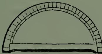
diameter of which a dot or small cut is made, indicating the centre; the edges are divided into 180 parts or degrees, or 360 parts or half degrees; the best protractors are always divided in half degrees. The horn protractors are made of a solid piece of horn, rolled as thin as
